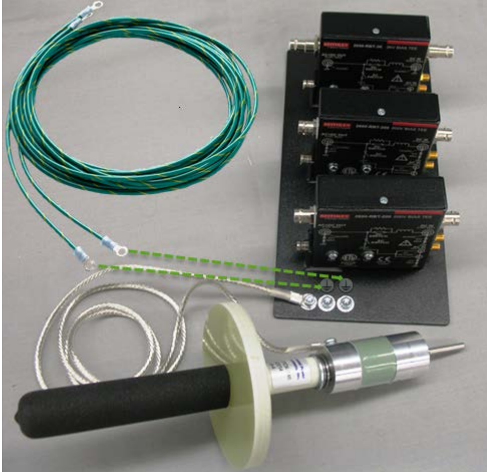
Figure 3: Bias tee mounting bracket with CA-568-120 grounding cable connection example
