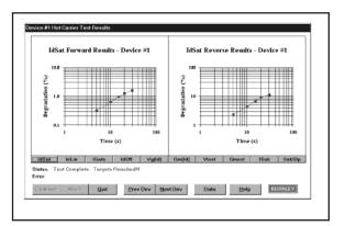
The Hot Carrier System provides results in real time. At any point during the test, the measured parameters for each device can be displayed numerically or graphically by clicking the status display. The status display also includes the time on stress and the time to next readpoint.
