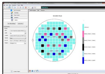
Wafer and binning map tools allow you to browse through the test results on either a wafer-by-wafer or site-by-site basis. You can also overlay traces from multiple sites to make quick comparisons.
