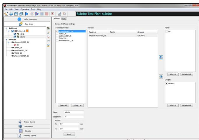
**ACS lets you map devices and tests to sites and subsites, eliminating the need to duplicate each test for each subsite and reducing your test development time significantly.**
