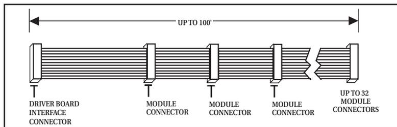
The METRABUS cable used to connect all METRABUS I/O modules to a METRABUS controller is available in standard and non-standard configurations for virtually any arrangement. (See page 550 for ordering details.)
