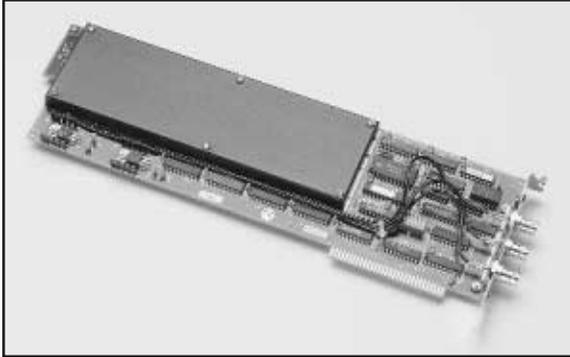
The PCIP-SCOPE features 2 input channels with real-time sample rates up to 20MHz and a bandwidth of 10MHz. For repetitive, high-speed signals, an interlace sampling mode increases the effective sample rate by as much as 25 times. You can use the trigger channel or either input channel to trigger via slope, level or under computer command. A 2048-sample memory is allocated to one channel or split evenly between two channels.
