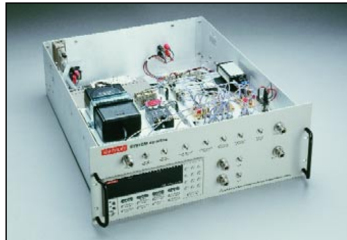
System 40 integrated with switches, attenuators, power dividers, and isolators
