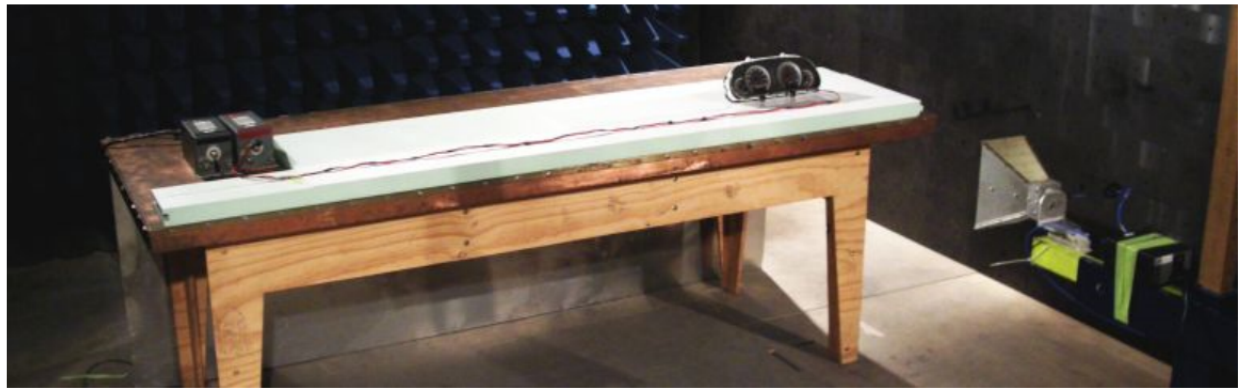
Photo: Above 1GHz CISPR 25 / EN 55025 type radiated emissions testing of an automotive driver display cluster
