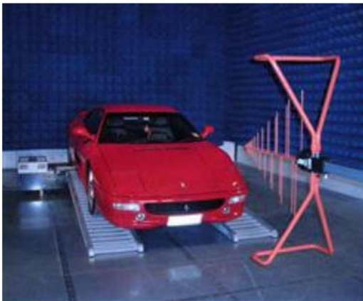
Photo: CISPR 12 / EN 55012 type testing
