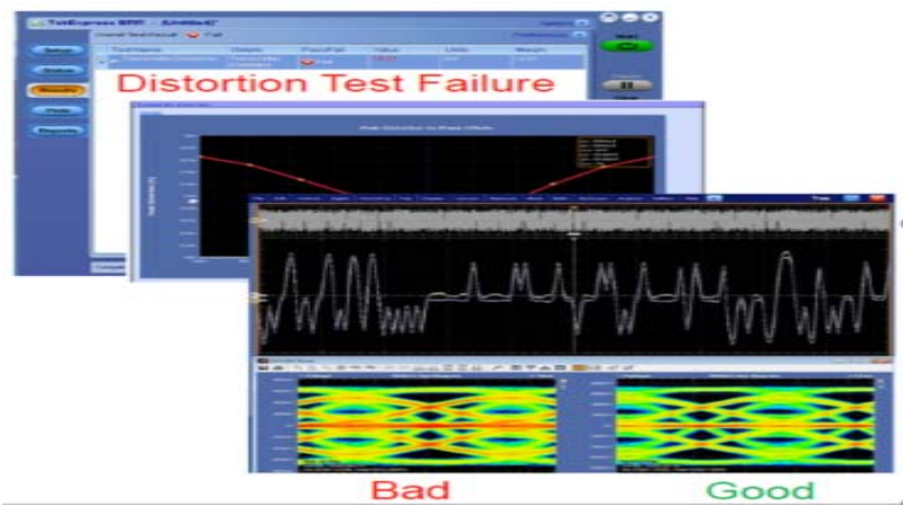
Timing error using DPOJET eye diagram
