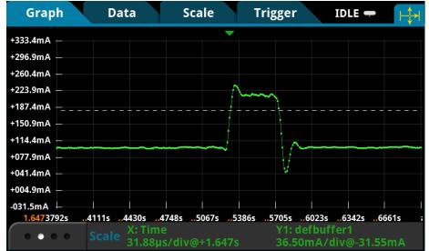
Detailed Power Consumption Profile using DMM7510
