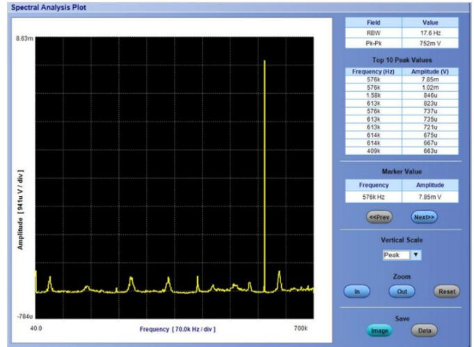
Figure 9. Spectral analysis plot of DC-DC converter.
