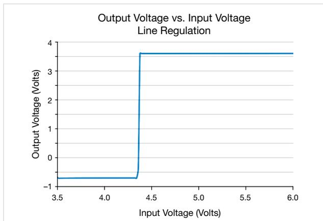
Figure 6. Plot of DC-DC converter line regulation measured using a single Model 2612B SourceMeter SMU instrument.
