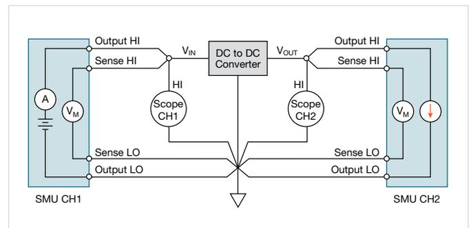
Figure 7. Testing a non-isolated DC-DC converter using both a scope and two SMUs.
