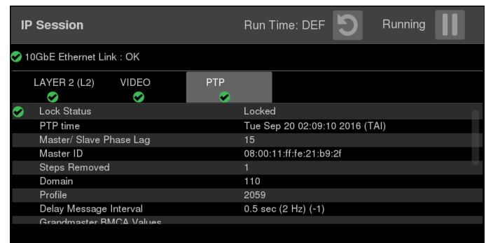
FIGURE 12. Monitoring PTP packet headers to ensure that devices are on the correct domain.
