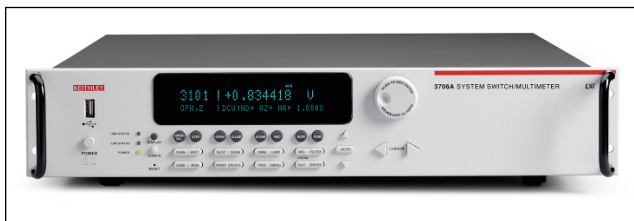
Figure 4. The Model 3706A System Switch/Multimeter supports up to 360 thermocouple channels in a single 2U chassis.
