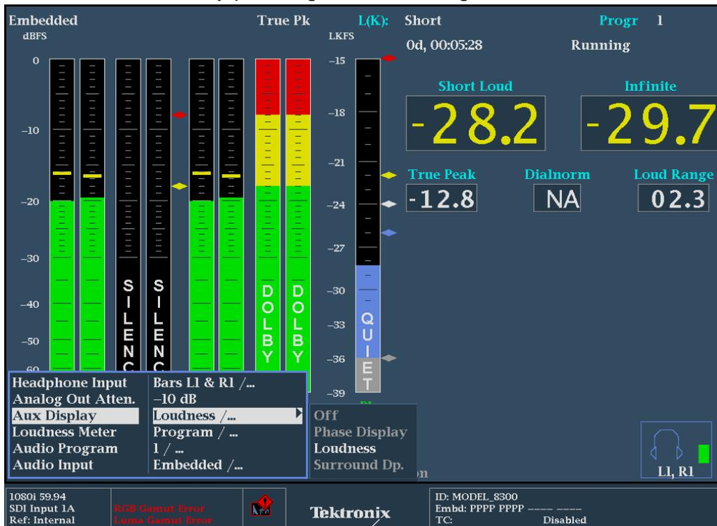
Figure 4. Loudness Readouts within Audio Display.
