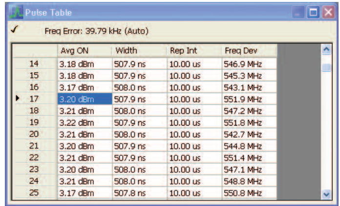
Figure 21. The Pulse Table on SignalVu vector signal analysis software showing the parameters of the 500 MHz chirp.
