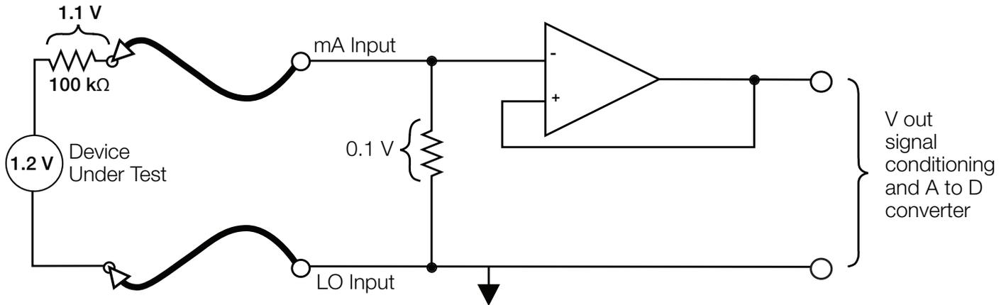
Figure 1. Circuitry of a shunt multimeter used as an ammeter.
