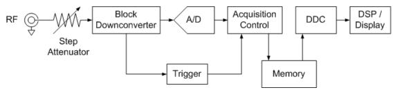
At the core of the MDO is the same Tektronix-proprietary A/D converter used in most Tektronix oscilloscopes. This 8-bit A/D converter samples at 10 GS/s and has an input bandwidth in excess of 5 GHz. In order to extend the input frequency response in the 6 GHz MDO models, a downconverter is used before the A/D. This downconverter supports the following input frequency ranges:
