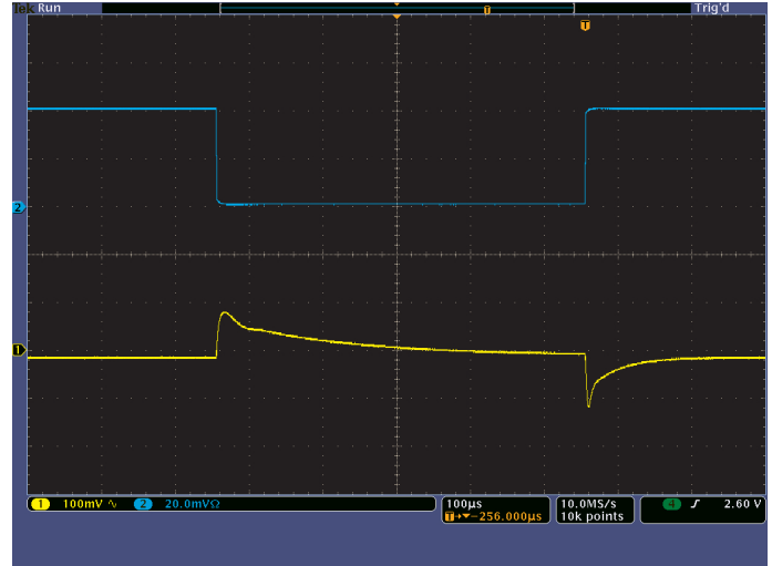
Figure 11. Dynamic load response of 5V output. Blue trace is current (20mA/Div) and yellow trace is voltage (100mV/Div).
