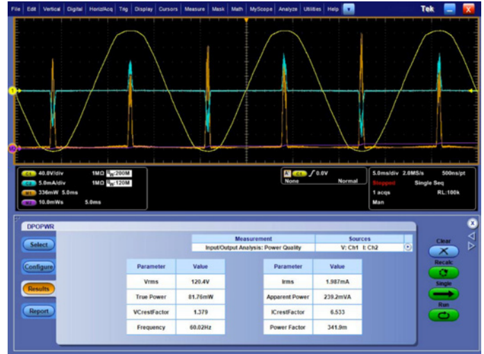
Figure 16. Power Quality Measurements on an unloaded Bluetooth pairing device charger.
