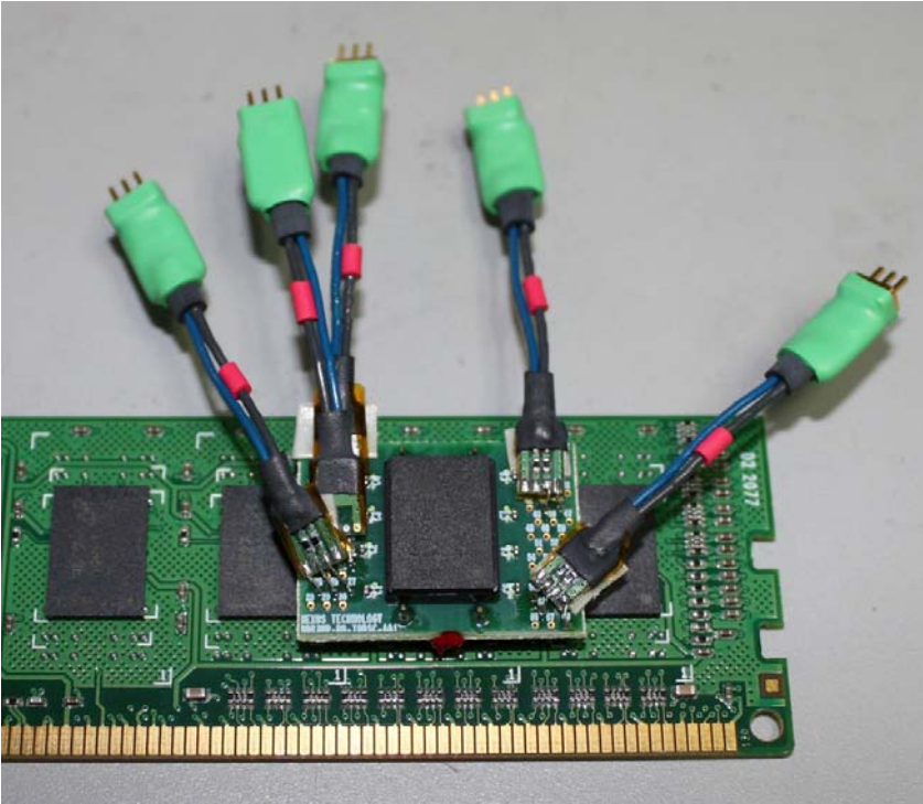
Figure 7. All tips soldered to DDR Component Interposer
