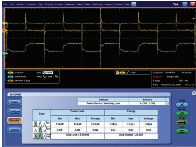
Figure 8. Switching Loss Measurements Using DPOWPR.
