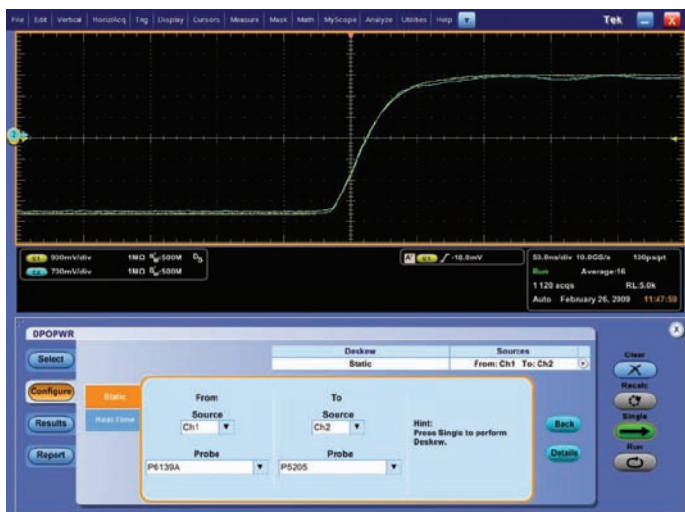
Figure 2. Static Skew Compensation Between Two Probes, AFTER Adjustment.
