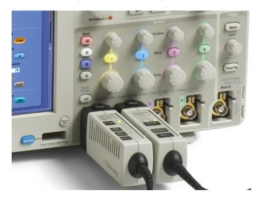
The internal power supplies of these oscilloscopes provide power to the TekVPI probe inputs located on the front of the oscilloscope (Channels 1, 2, 3, 4, Aux In, and RF). Because some of the available TekVPI probes can draw a significant amount of power, it is possible that multiple probes may exceed the oscilloscope's available internal power.
