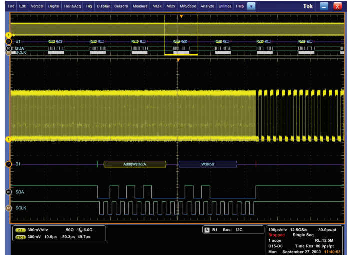
Figure 2. MSO70000 Series can provide time correlated views of analog and digital signals.
