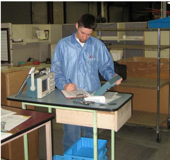
Figure 3: Incoming instruments are logged in, entered into the tracking system, and checked for physical damage.
