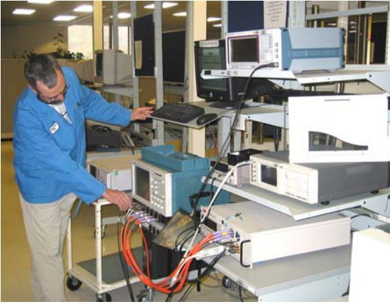
Figure 5: Setting up an automated calibration for a high-performance oscilloscope.
