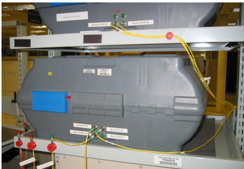
Figure 7: Just another piece of luggage? No, this is a test fixture containing more than 200 kilometers of singlemode optical fiber cable.
