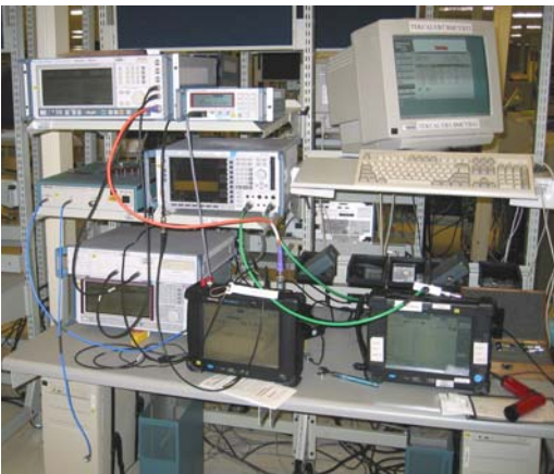
Figure 6: The compact, portable NetTek analyzer requires a bench-full of calibration equipment.
