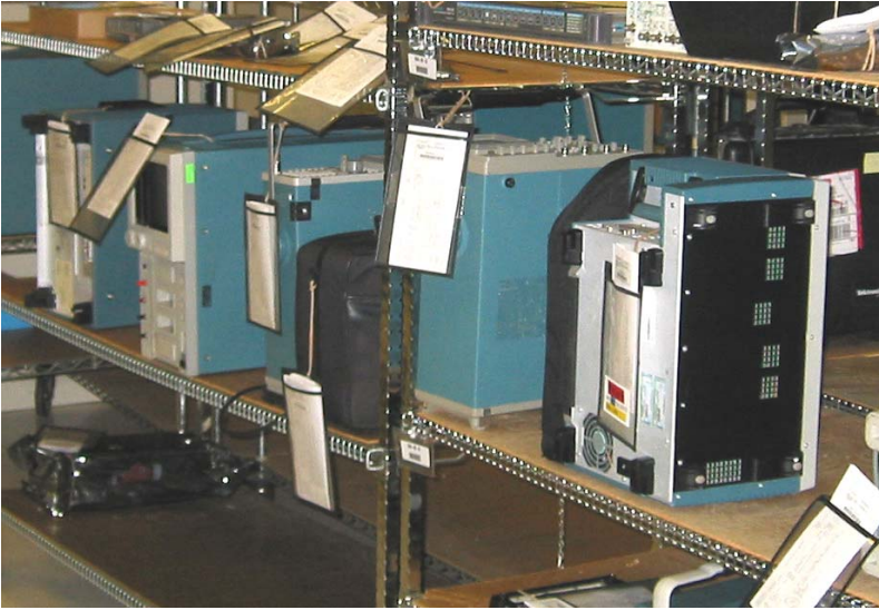
Figure 4: Instruments are tagged and queued for calibration.
