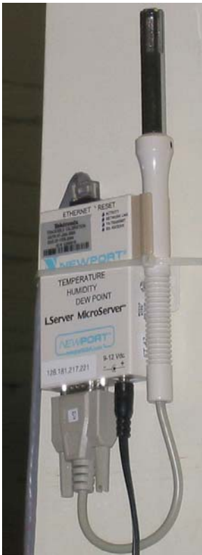
Figure 9: Temperature and humidity sensors keep environmental conditions within standard limits, and protect against static electricity buildup.
