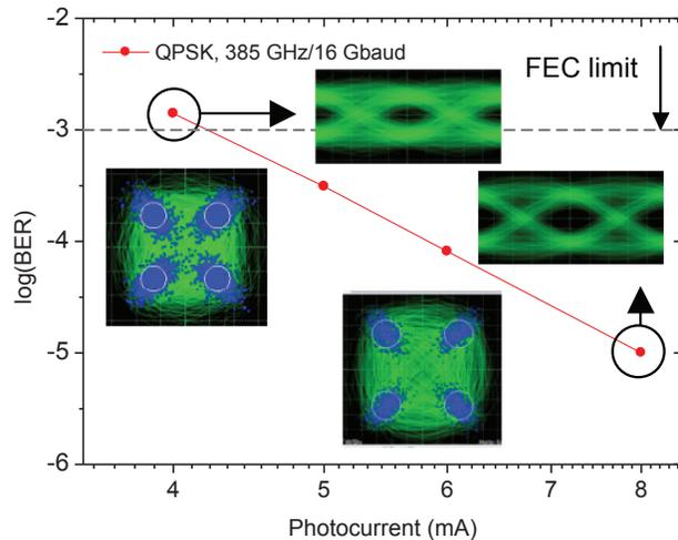
Figure 5: BER curves measured for the 16 GBaud (32 Gbit/s) QPSK signal (0.65 Gaussian filtering). Insets show the constellation diagrams (blue points: sampling points) and eye diagrams.
