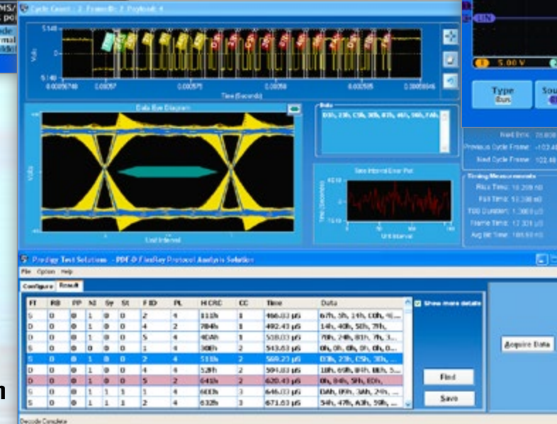
DP04AUTOMAX Eye Diagram analysis of a FlexRay signal.
