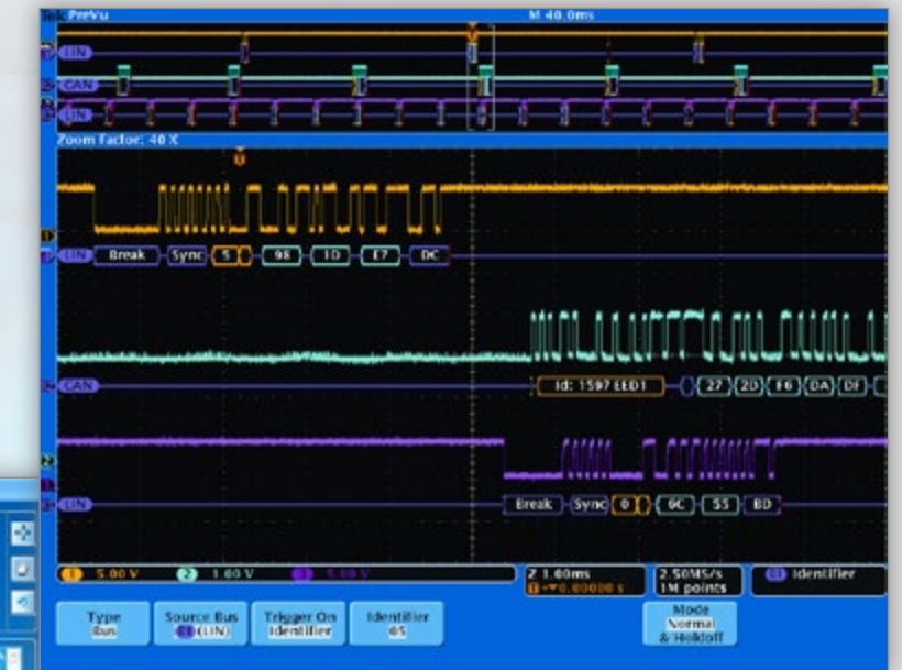
Simultaneous capture and decode of multiple automotive serial buses.
