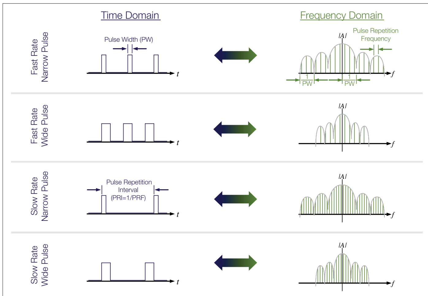
Figure 6. Spectrum plot measurements of pulse width and repetition rate.
