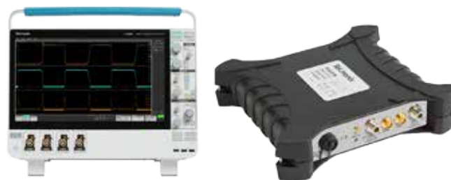
Figure 3. The 5 Series MSO and RSA500 can be used together to perform multiple domain measurements.
