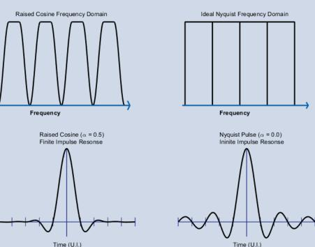
Frequency Domain (above) and Time Domain (below) representation of a raised cosine filter. Left signal has a roll-off factor of 0.5, leading to a finite impulse response, while the right has a roll-off factor of 0 leading to an infinite impulse response.
