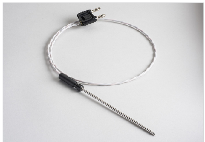
Figure 14. Thermocouple temperature transducer.
