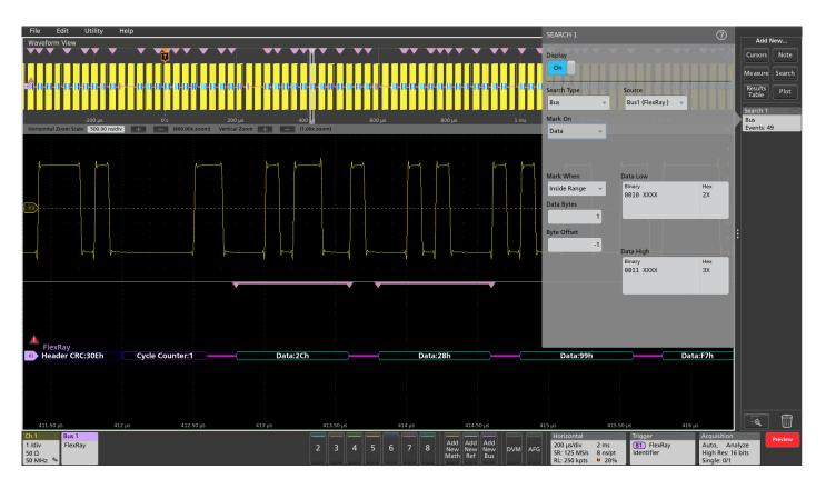
But how many of the events occurred? To find all of the bus events that meet a specific search criteria, you can use automated Wave Inspector search. The setup is similar to the bus trigger setup, allowing the oscilloscope to find and mark all of the specified bus events.
