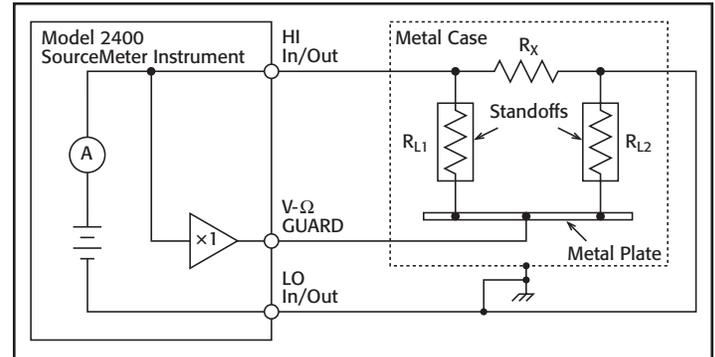
Figure 5. Model 2400's Built-In Guard.
