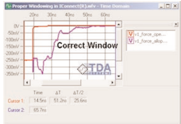
Figure 15. Proper windowing of the TDR waveform for further analysis in IConnect TDR software. The properly windowed waveform will exclude the first transition, corresponding to the interface between the TDR sampling head to the cable, but will keep the window sufficiently long to allow all the reflections corresponding to the DUT, to be included in the window
