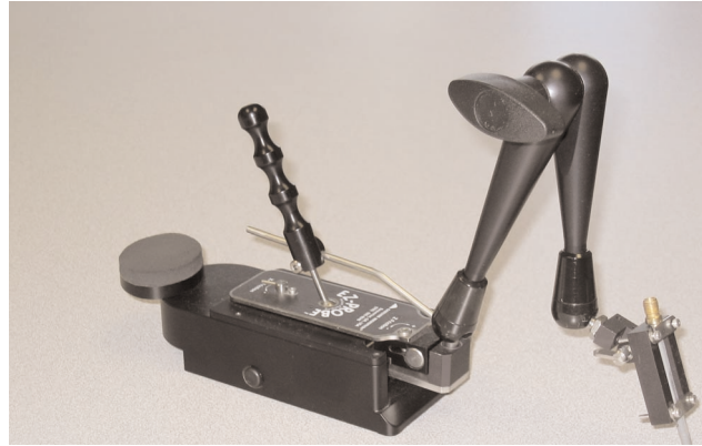
Figure 13. TDA Systems QuickTDR™ probe supported by Cascade Microtech EZProbe™ positioner. The spacing between signal and ground in the tip of the probe is extremely small to ensure best performance
