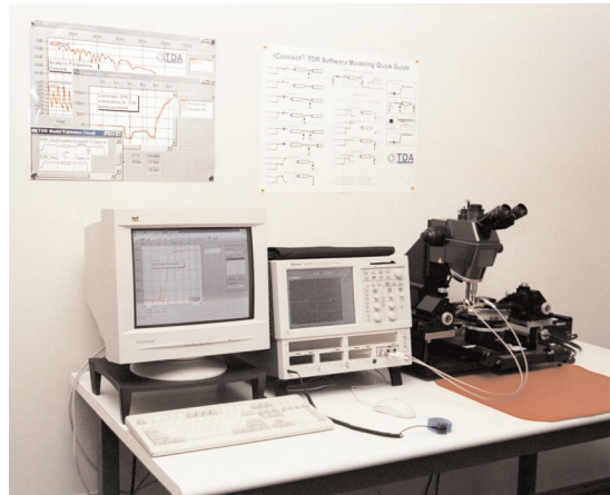
Figure 2. A typical failure analysis setup includes a TDR instrument, a probing or fixturing setup, and analysis software
