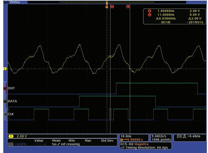
Figure 18. Clock glitch caused by non-monotonic rising clock edge.
