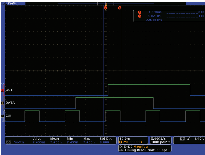
Figure 16. D-Flip-Flop operation looks normal based on one acquisition.
