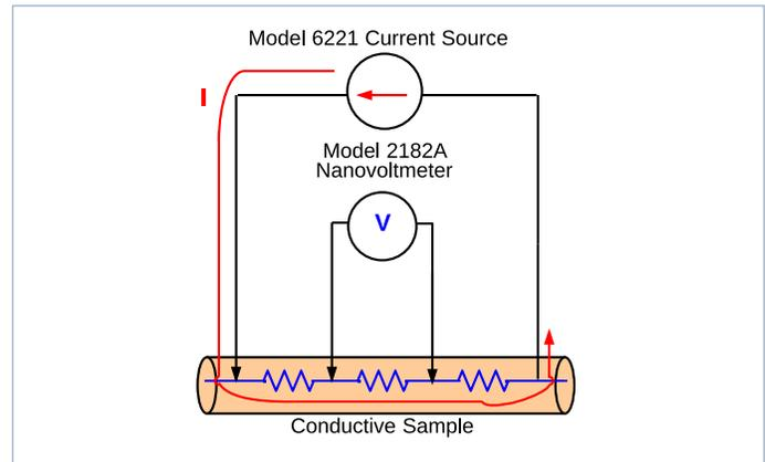
Figure 5. Using a current source and nanovoltmeter to measure a conductive sample.
