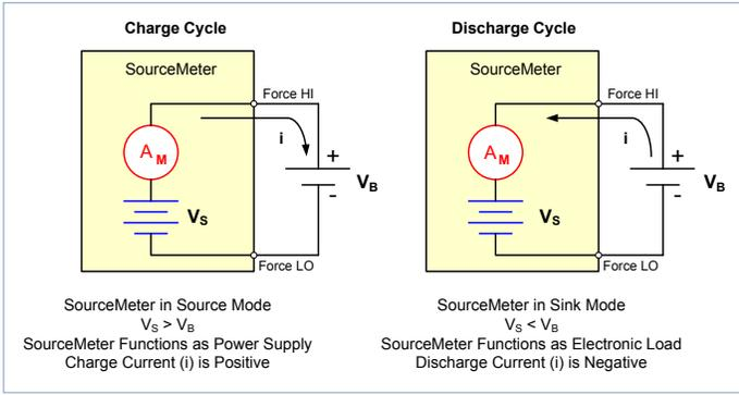
Figure 13. Charge and discharge circuit diagrams.
