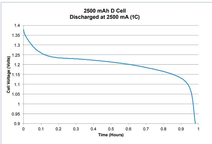
Figure 14. Discharge characteristics of 2500 mAh D cell battery using Model 2460.
