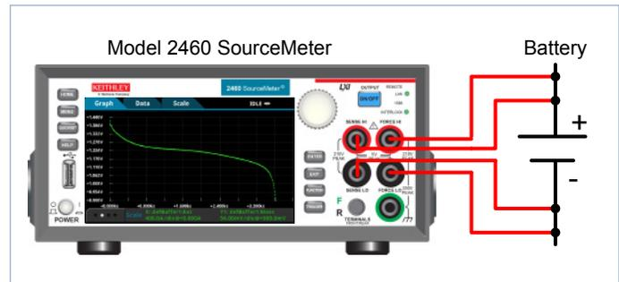
**Figure 12.** Results of discharging battery shown on graphical display of Model 2460 SourceMeter SMU instrument.
