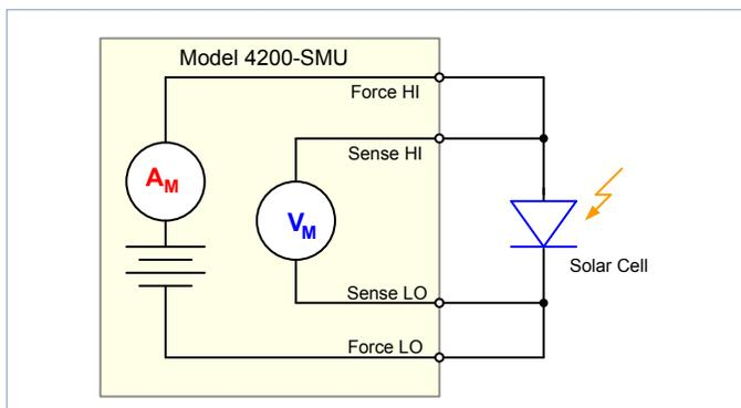
**Figure 10.** A solar cell connected to a Model 4200-SMU Parameter Analyzer.
