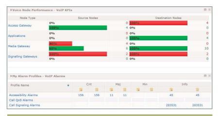
Drag and drop portlets allow each user to focus on specific areas of responsibility. In this example, Node performance is reported against user-defined thresholds while a running tabulation of VoIP alarms and severity is featured in the portlet below.
