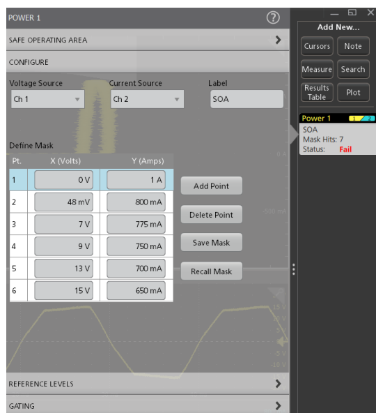
FIGURE 7. SOA Mask Editor window. The mask is defined by a set of (voltage, current) coordinates taken from the switching device datasheet, or may be user-defined.
