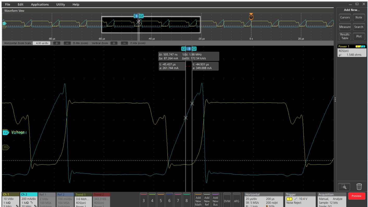
FIGURE 10. RDS(on) measurement. The Ch1 (yellow) waveform is the FET V_{DS} voltage and the Ch2 (cyan) waveform is the FET current. The waveforms are inverted in phase to correctly indicate that the current is high in the conduction region. The results badge (upper right) shows the mean RDS(on) value by default, but can also be configured to show the minimum value. In this example, cursor gating is being used to find the minimum RDS(on) value, which is typically close to an ohm (1.58 ohms in the figure).
