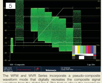
waveform mode that digitally recreates the composite signal waveform from the digital input. This feature allows the operator to visualize the familiar composite signal.
