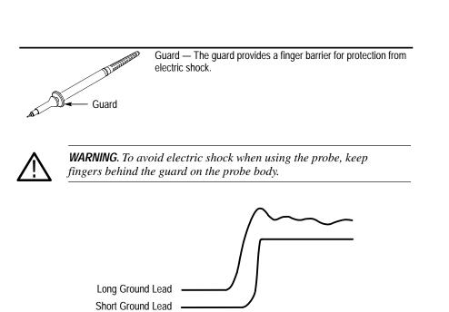
To see the best signal, use the shortest possible ground lead and signal path.
