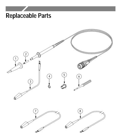
Figure 3: P6119B Replaceable Parts
