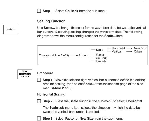
The magnification for scaling can be set with either Factor or New Size.
