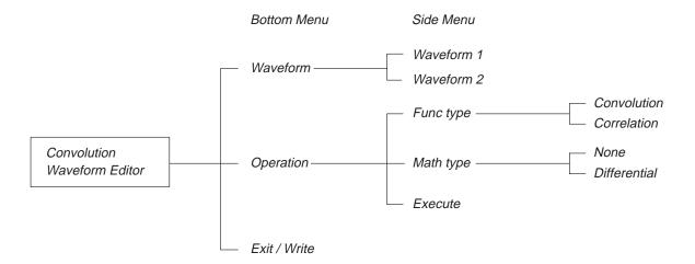
Figure 4A-152: Convolution Waveform Editor Menu Structure
