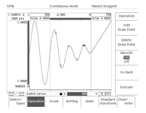
Figure 2-34: Connecting the Points
