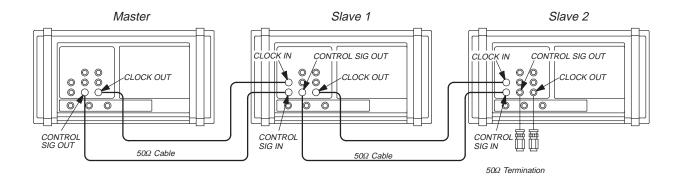
Figure 4C-9: AWG2005 Parallel Operation
