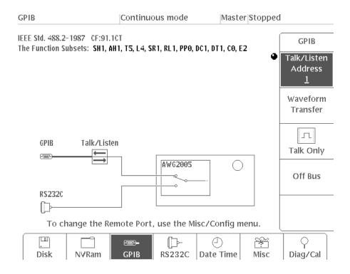
Figure 4E-9: Menu Displayed When GPIB is Selected
