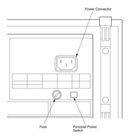
Figure 1-1: Rear Panel Controls Used In Start Up
