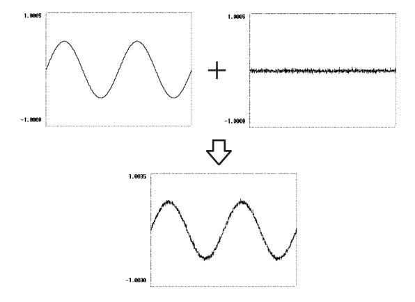
Figure 4A-21: Adding Noise to the Sine Wave
