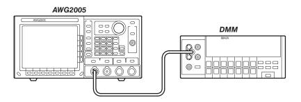
Figure E-14: Gain Accuracy Initial Test Hookup
