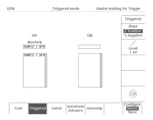
Figure 2-55: Menu Displayed When Triggered is Selected
