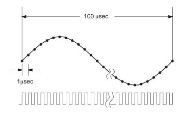
Figure 4B-4: Clock and Waveform Points
