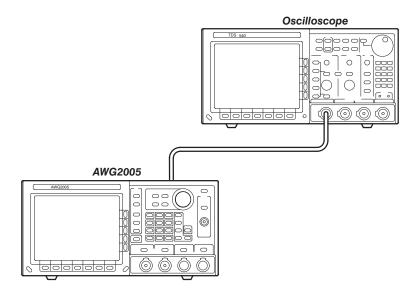
Figure E-13: Clock Amplitude Initial Test Hookup
