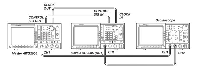
Figure E-21: Slave Operation Initial Test Hookup
