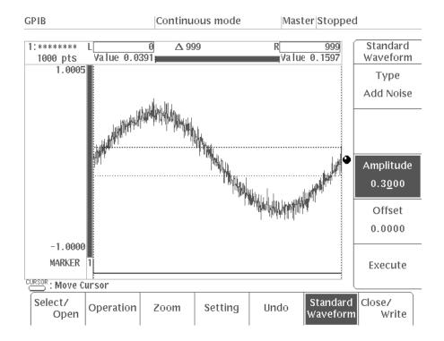
Figure 2-36: Sine Wave With Noise Added
