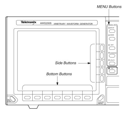
Figure 2-7: Menu Buttons and Bezel Buttons
