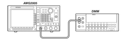
Figure E-15: Offset Accuracy Initial Test Hookup
