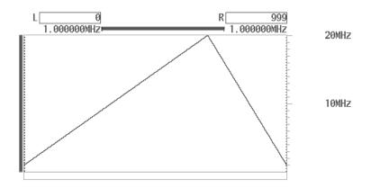
Figure 4A-148: Creating a Linear U/D Clock Sweep
