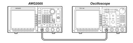
Figure E-16: Pulse Response Initial Test Hookup
