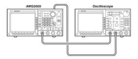
Figure E-9: Autostep Mode Initial Test Hookup
