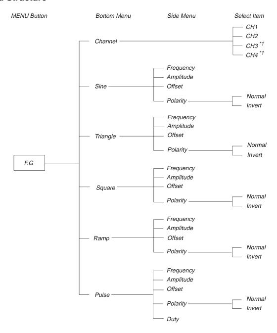
Figure 4F-1: FG Mode Menu Structure
