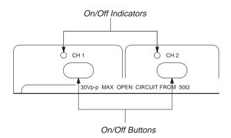
Figure 2-23: Channel On/Off Buttons and Indicators
