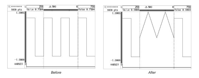
Figure 4A-47: Integral Calculation
