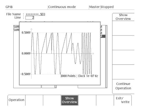
Figure 2-43: Sequence Waveform Display With Show Overview Selected
