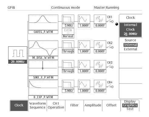
Figure A-1: SETUP Menu for 4-Channel Display
