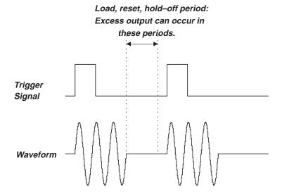
Figure A-7: Generation of Excess Output
