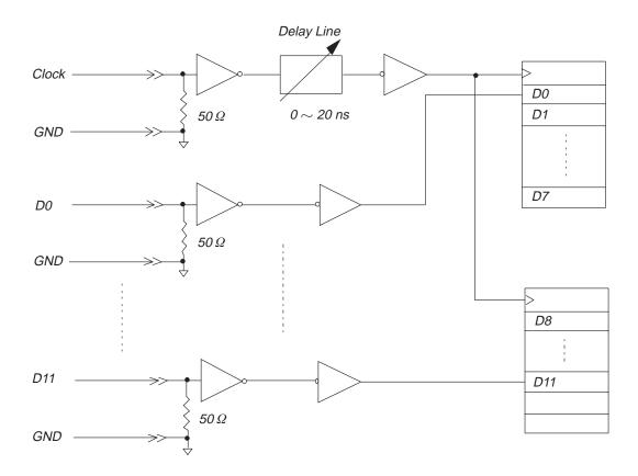
Figure A-12: Waveform Reproduction Circuit Example
