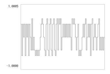
Bit rate 42 Kbps Point number 32 Kwords Clock frequency 21 kHz
