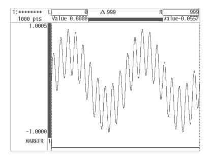
Figure 4A-52: Waveform Addition Display
