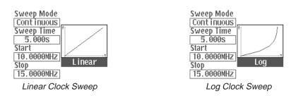
Figure 4B-13: Sample Linear and Log Clock Sweep Settings
