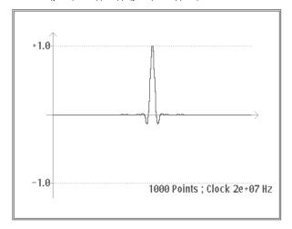
Figure C-6: Nyquist Pulse Formula and Waveform
