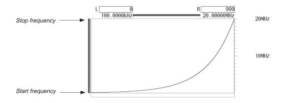
Figure 4A-143: Sample Log Clock Sweep
