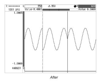
Figure 4A-33: Vertically Inverted Display
