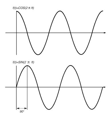
Figure D-6: Phase and Delay
