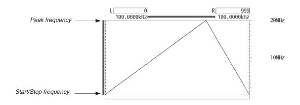
Figure 4A-144: Sample Linear U/D Clock Sweep
