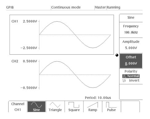
Figure 2-68: CH1 Output Parameter Setting Display
