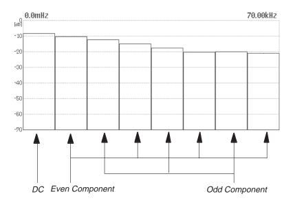
Figure 4A-167: Fundamental, Odd, and Even Components
