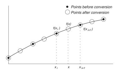
Figure D-1: Linear Interpolation
