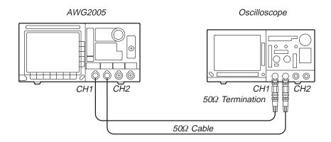
Figure 2-70: Connections for Example 6
