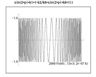
Figure C-10: Frequency Modulation Formula and Waveform
