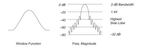
Figure D-9: Hanning Window and Frequency Characteristic
