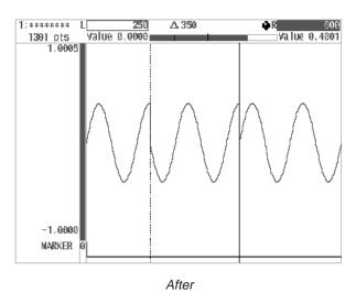
Figure 4A-32: Horizontally Inverted Display
