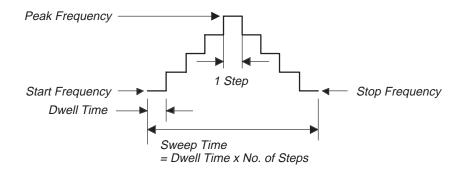
Figure 4A-137: Sample Linear Up/Down Clock Sweep Waveform
