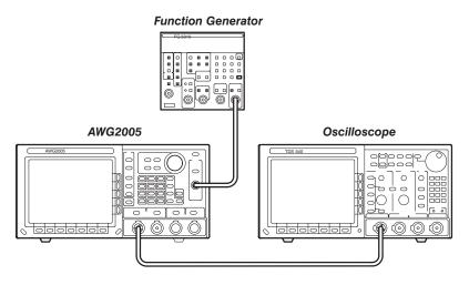
Figure E-19: External Trigger Level Accuracy Initial Test Hookup
