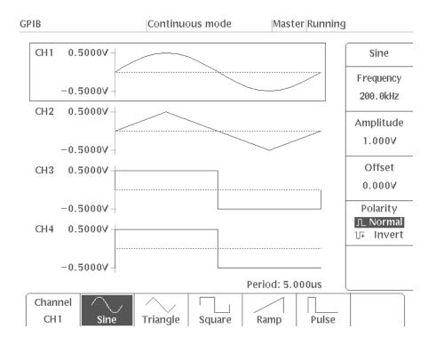
Figure A-3: FG Menu for 4-Channel Display
