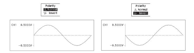
Figure 4F-5: Waveform Polarity
