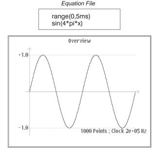
Figure 4A-96: Example of Equation File Data and Resulting Waveform
