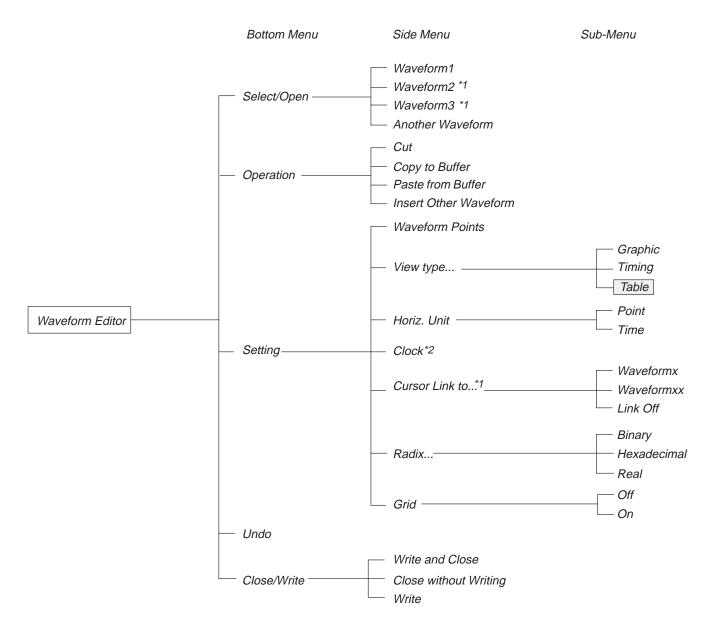
Figure 4A-93: Waveform Editor Table Display Menu Structure
