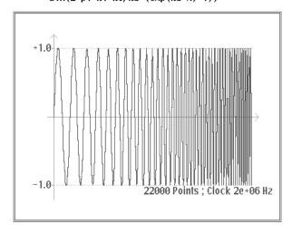
Figure C-8: Log Frequency Sweep Formula and Waveform
