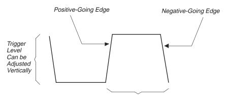
Trigger Slope Can be Positive or Negative
