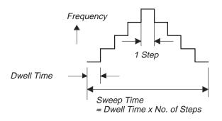
Figure 4B-14: Arbitrary Clock Sweep Waveform
