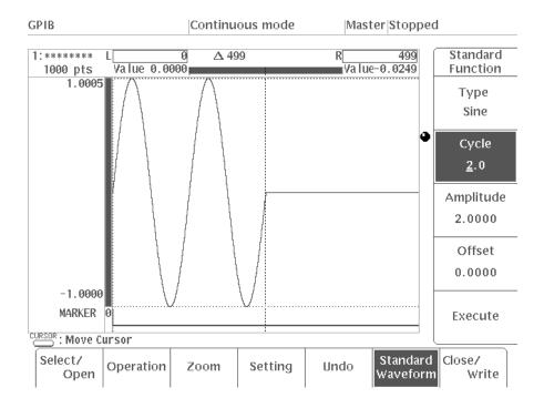
Figure 2-27: Creating a Sine Waveform
