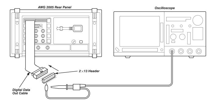
Figure E-22: Digital Data Out Initial Test Hookup
