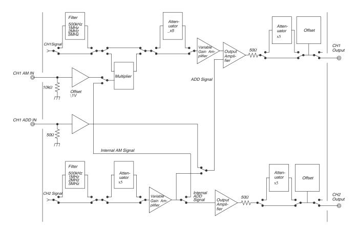
Figure 3-8: Block Diagram of the Analog Circuit
