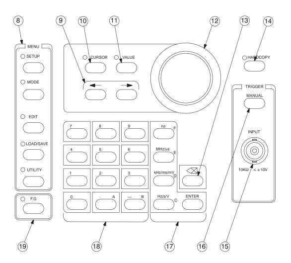
Figure 2-2: Front Panel Button Detail
