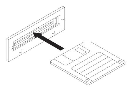
Figure 2-15: Inserting the Floppy Disk
