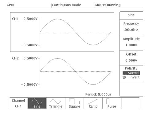
Figure 2-67: Screen When Sine Set for CH1
