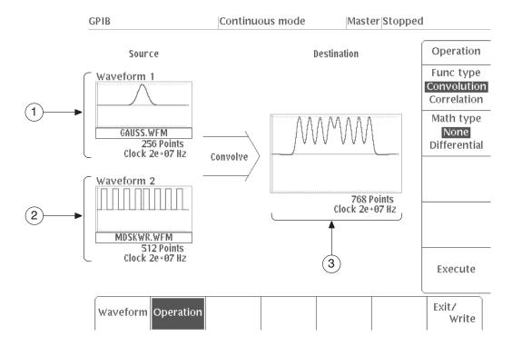
Figure 4A-153: Convolution Waveform Editor CRT Display
