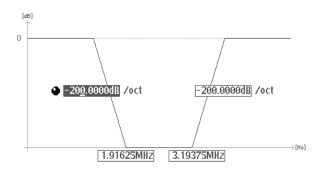
Figure 4A-166: Band Cut Filter
