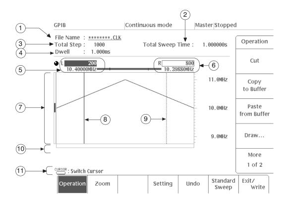
Figure 4A-139: Clock Sweep Editor CRT Display
