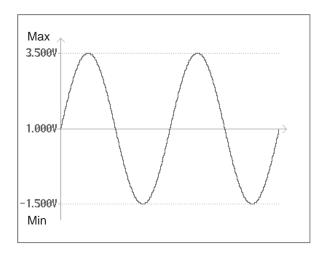
Figure 4B-9: Amplitude and Offset Setting
