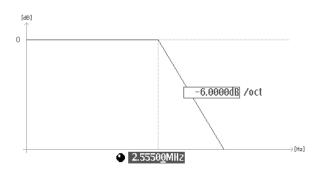
Figure 4A-163: Low Pass Filter
