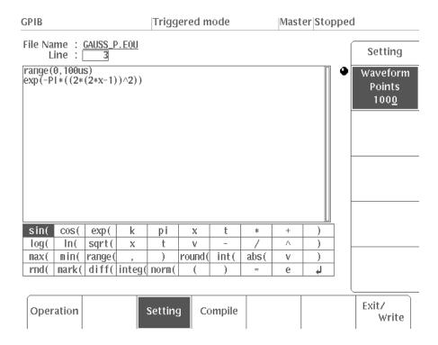
Figure 4A-117: Setting Waveform Point Count
