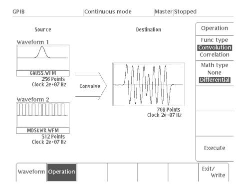
Figure 4A-155: Sample Convolution
