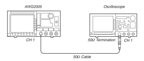
Figure 2-22: Connections in Example 2
