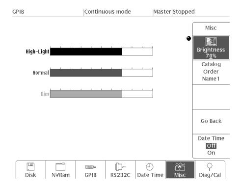
Figure 2-14: Setting the Display Brightness
