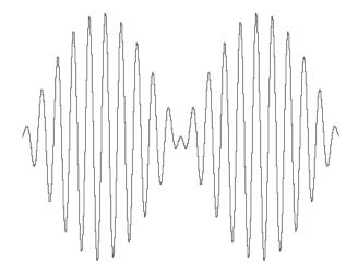
Figure 3-9: 100% Amplitude Modulation
