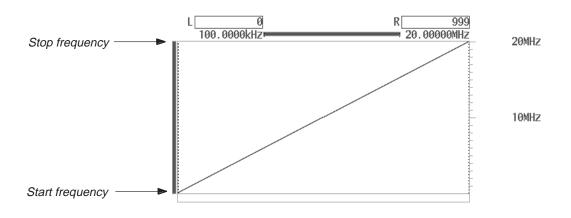
Figure 4A-142: Sample Linear Clock Sweep
