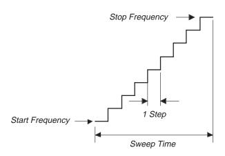
Figure 4B-12: Linear Clock Sweep Waveform
