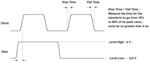
Skew : Measure at 50% level of the waveform : must be no greater than  $\pm$  15 ns.
