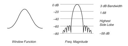
Figure D-12: Blackman Window and Frequency Characteristic
