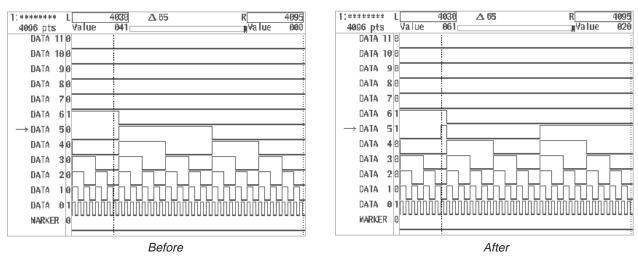
Figure 4A-85: Inverting Waveform Data State
