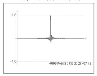
Figure C-3: Sampling Function SIN(X)/X Pulse Formula and Waveform
