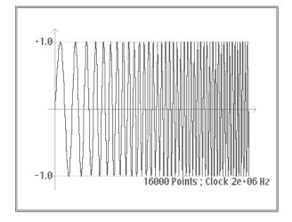
Figure C-7: Linear Frequency Sweep Formula and Waveform
