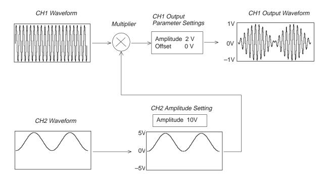
Figure 4B-5: Multiplying CH1 Waveform by CH2 Waveform
