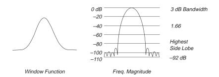
Figure D-11: Blackman-Harris Window and Frequency Characteristic
