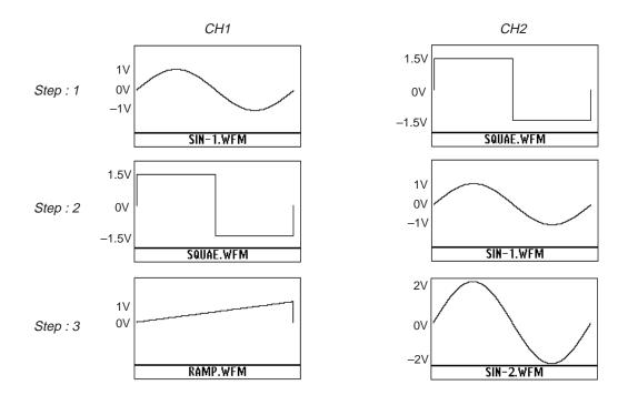
Figure 4A-125: Autostep File Data and Output Waveforms
