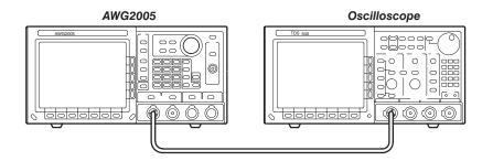
Figure E-4: Cont Mode Initial Test Hookup
