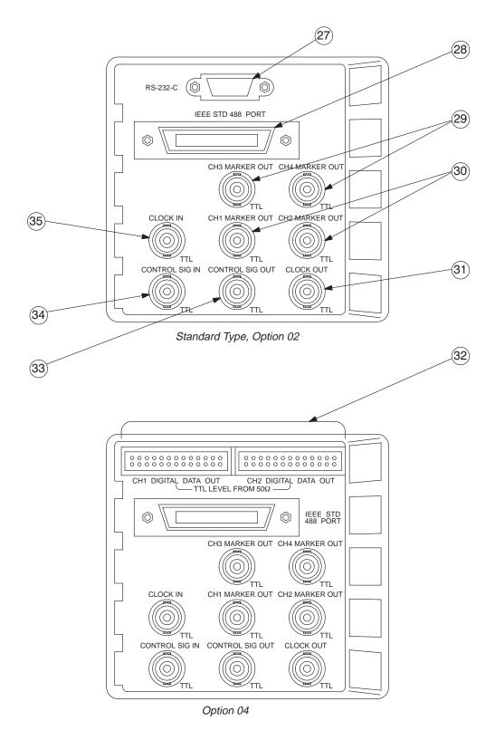
Figure 2-5: Rear Panel Detail
