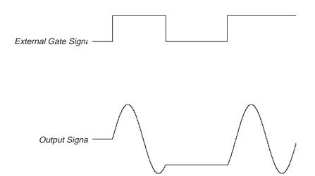
Figure 4C-4: Output Waveform for External Gate Signal in Gated Mode
