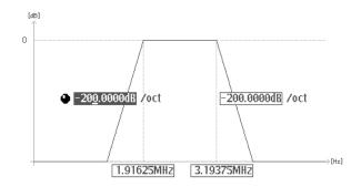
Figure 4A-165: Band Pass Filter
