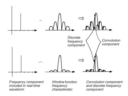
Figure D-7: Concept of Convolution
