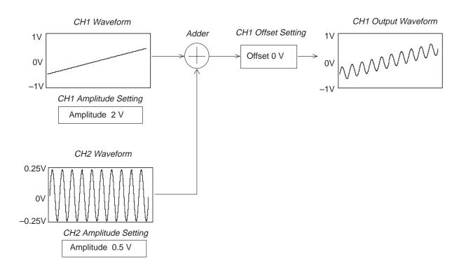
Figure 4B-6: Adding CH1 Waveform and CH2 Waveform
