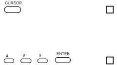
Step 3: Press the front panel CURSOR button to activate the right side vertical bar cursor (it becomes a solid line).
