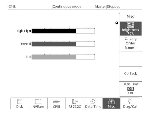
Figure 4E-12: Setting the Display Brightness
