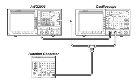
Figure E-6: Gated Mode Initial Test Hookup
