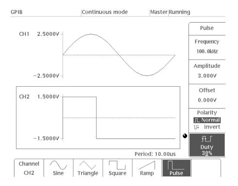
Figure 2-69: CH2 Output Parameter Setting Display
