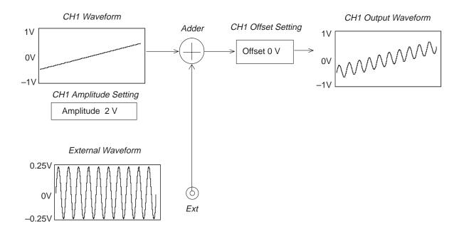
Figure 4B-8: Adding CH1 Waveform and External Waveform
