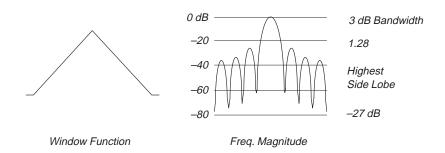
Figure D-13: Triangle Window and Frequency Characteristic
