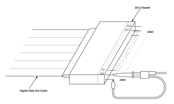
Figure E-23: Output Pins on the Digital Data Out Cable
