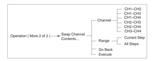
Autostep files created on instruments with Option 02 installed may have files set for CH3 and CH4. In such cases, it is possible to swap step contents with CH3 or CH4.
