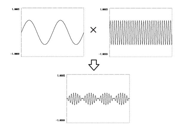
Figure 4A-22: Multiplying Sine Waves
