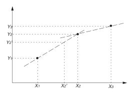
Figure 4A-55: Linear Interpolation
