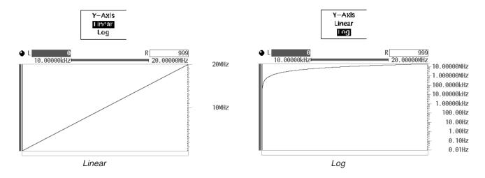
Figure 4A-140: Y-Axis Scale Settings
