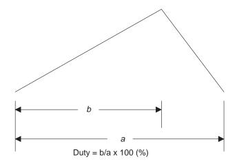
Figure 4A-147: Duty for U/D Clock Sweep
