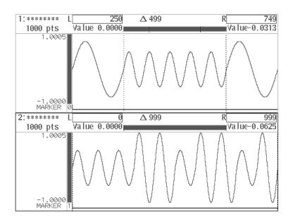
Figure 4A-66: Waveform Copying (number of points in waveform > Interval value)
