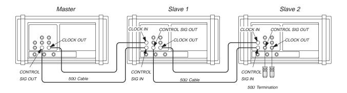
Figure 3-3: Connecting Three AWG2005 Instruments in Parallel
