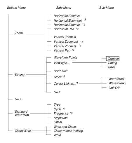
Figure 4A-14: Waveform Editor Graphic Display Menu Structure
