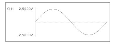
Figure 4F-3: Setting the Amplitude
