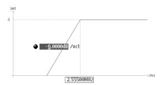
Figure 4A-164: High Pass Filter
