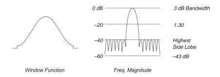
Figure D-10: Hamming Window and Frequency Characteristic
