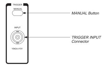
Figure 2-56: MANUAL Button and TRIGGER INPUT Connector
