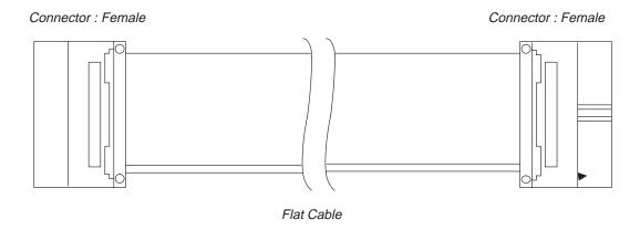
Figure A-11: Digital Data Out Cable
