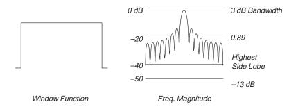
Figure D-8: Square Window and Frequency Characteristic
