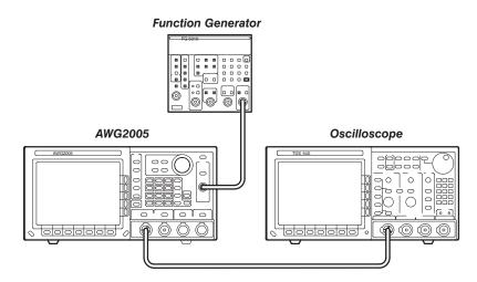
Figure E-5: Triggered Mode Initial Test Hookup
