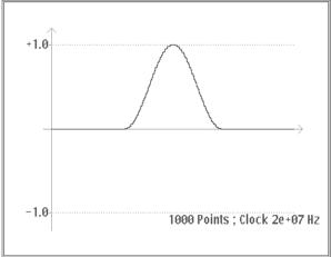
Figure C-4: Squared Sine Pulse Formula and Waveform
