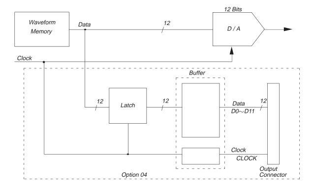
Figure A-5: Block Diagram
