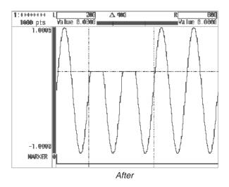
Figure 4A-34: Display of Waveform Clipped Above Clip Level
