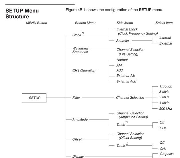
Figure 4B-1: SETUP Menu Structure
