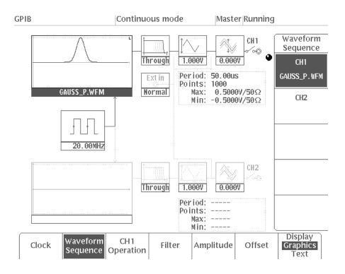
Figure 2-20: GAUSS\_P.WFM File Output Parameters
