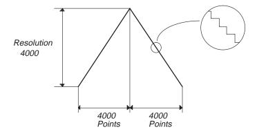
Figure 3-7: Relationship Between Triangular Wave Resolution and Number of Data Points
