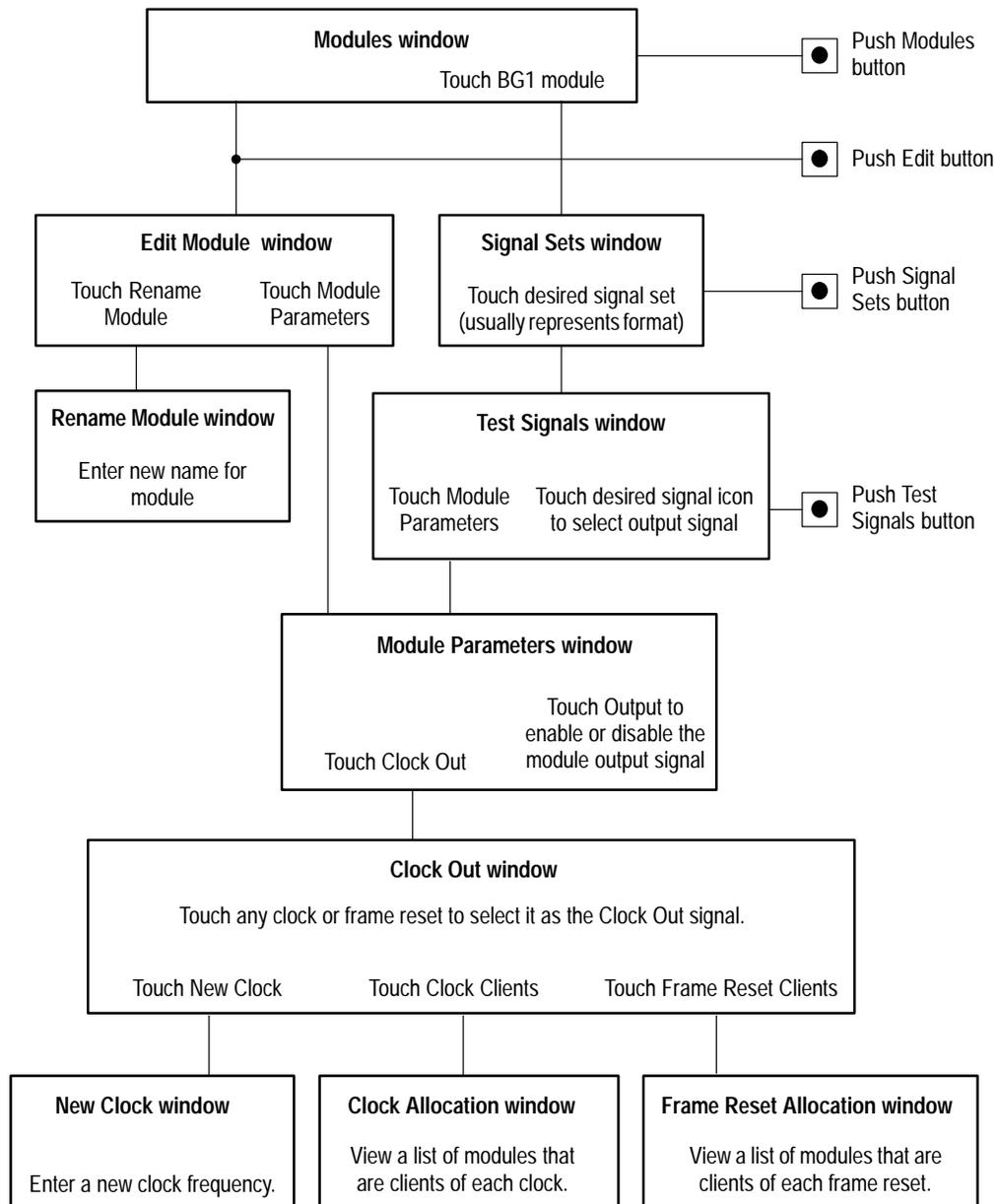
Figure 2–1: Basic menu structure for the BG1 Generator module
