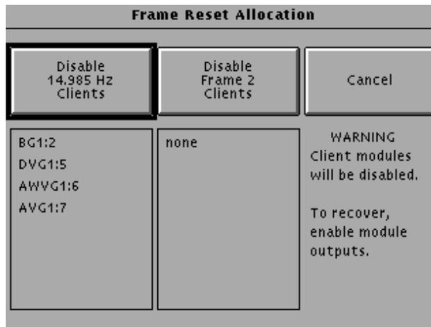
3. The Frame Reset Allocation window displays a list of all clients for each frame reset pulse. In the example, the BG1, DVG1, AWVG1 and AVG1 modules are using frame reset 1 which is set for 14.985 Hz. Frame 2 is unused.
