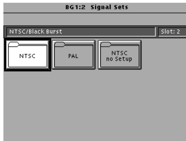
4. The Test Signals window for the selected signal set appears, as shown in the following illustration. In this example, the Black Burst signal is active. Change to another signal by touching the signal icon.
