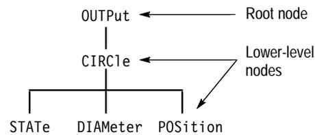
**Figure 3–1: Example of SCPI subsystem hierarchy tree**
