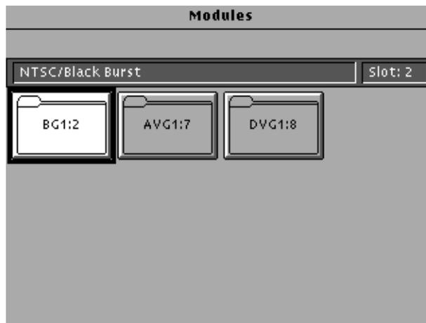
6. Touch the **BG1** icon on the display (or push the **Signal Sets** button if the BG1 icon is already highlighted). The installed signal sets for the module appear. Selections you make after this will pertain to the BG1 Generator module.
