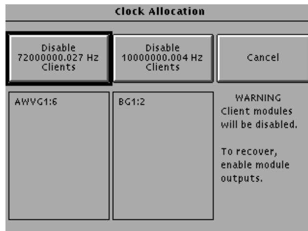
3. The Clock Allocation window displays a list of all clients for each clock. In the example, the AWVG1 module is using variable clock 1 which is set for 72 MHz, and the BG1 module is using variable clock 2 which is set for 10 MHz.
