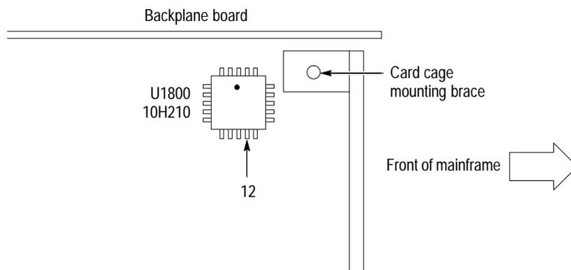
**Figure 3: Controller Board 100 MHz Time Base Clock Test Point Location (DAS 9221/TLA Mainframes)**
