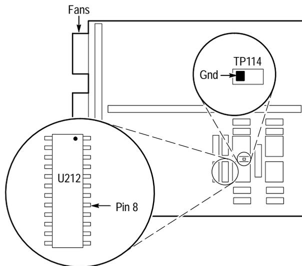
**Figure 7: 92HS8 Memory Board Test Point Locations (back of board)**
