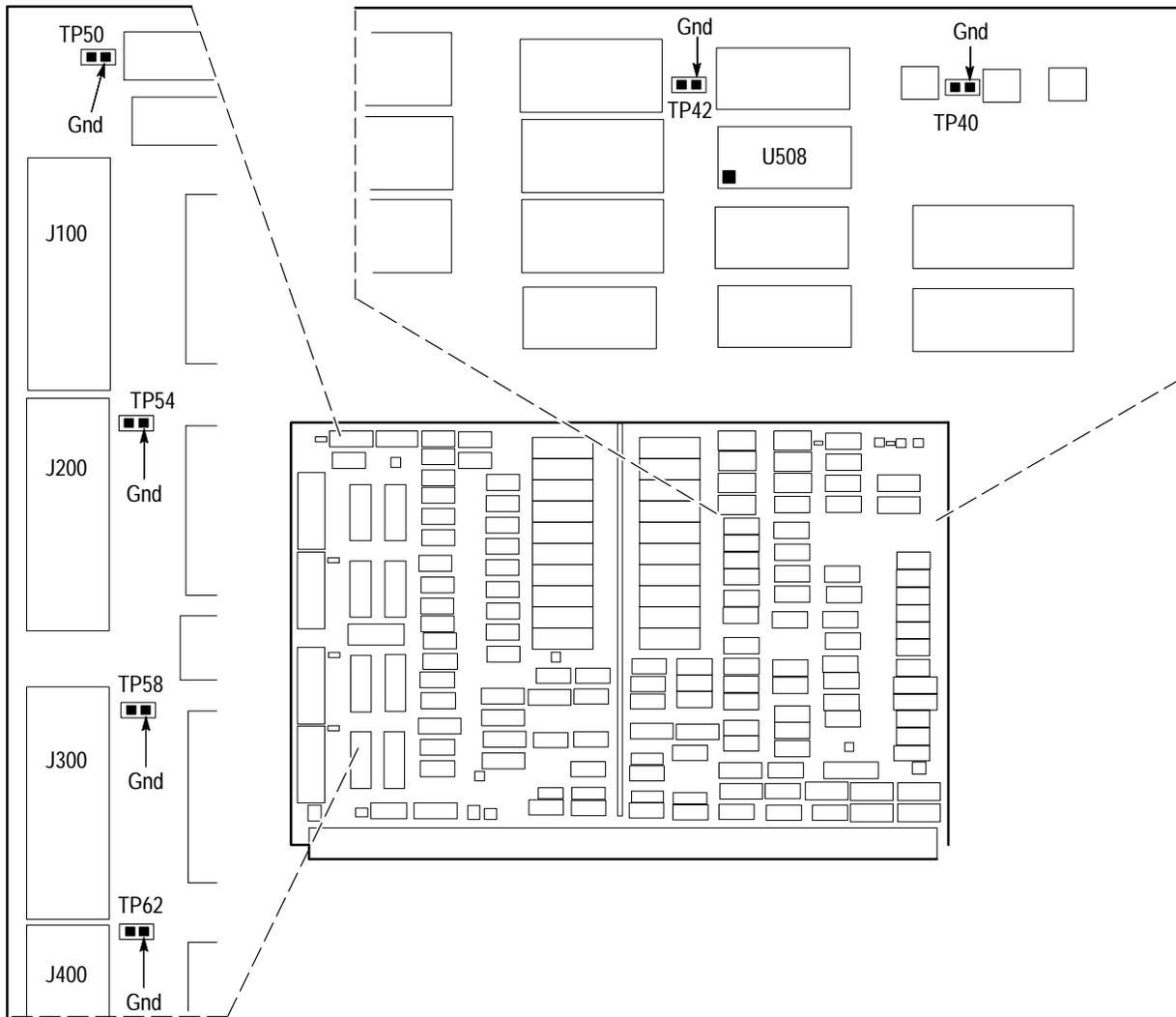
Figure 10: 92S32 Test Point Locations
