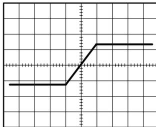
6. Using the Ch 1 probe, observe the signals at each test point listed in Table 4. Note how far the crossing points shift left (-) or right (+) of REF, and record the maximum value in each direction.
