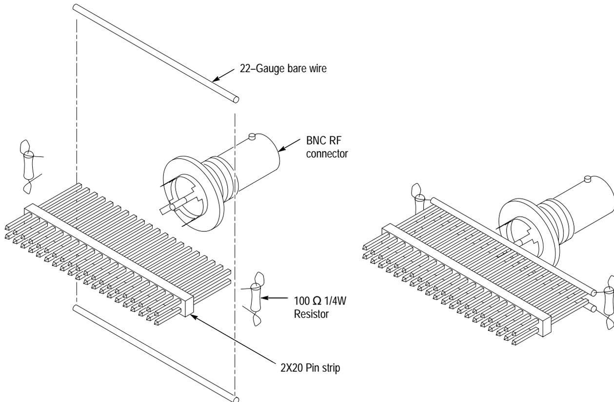
**Figure 11: 92A96 Acquisition Fixture Construction**
