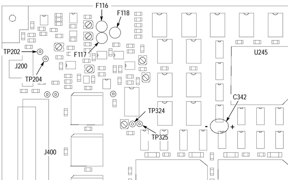
**Figure 6: Data and Clock Threshold Test Point Locations**
