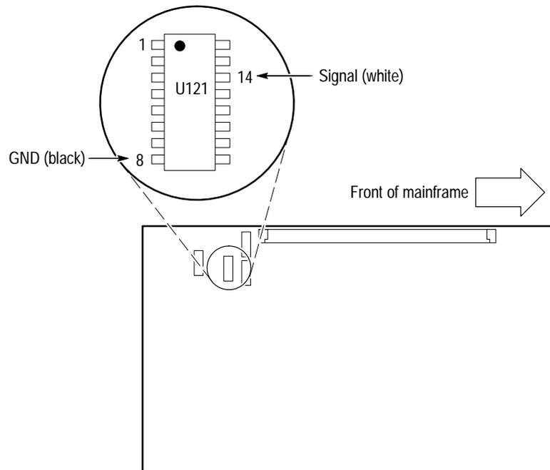
**Figure 2: Controller Board 100 MHz Time Base Clock Test Point Locations
