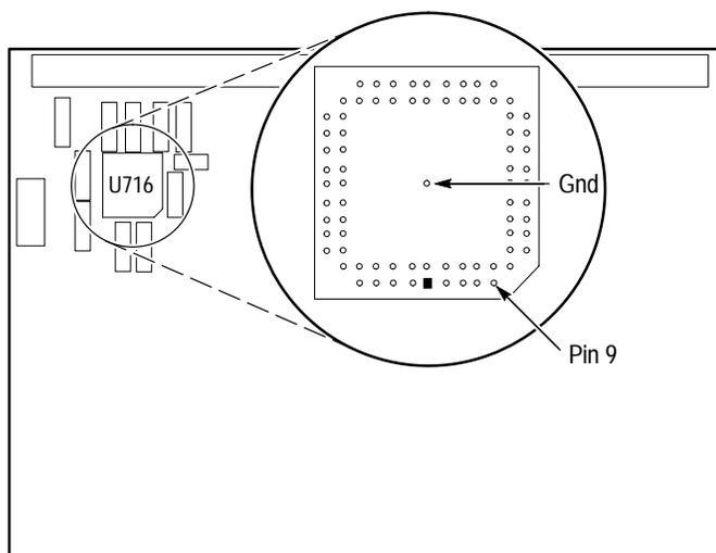
**Figure 5: 92A16 Test Point Locations (back of board)**
