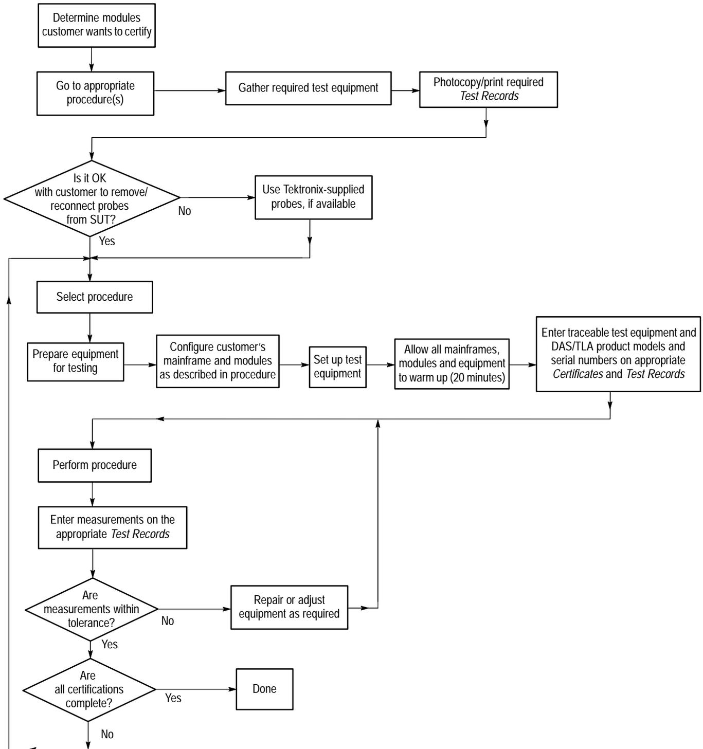
Figure 1: Certification Procedure Tasks
