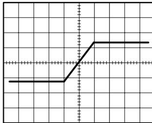
7. Probe TP156 using the Ch 1 probe. (See Figure 9 on page 57.) Note how far the crossing point of the rising edge has shifted to the right (+) or left (-) of REF. This is the skew value.
