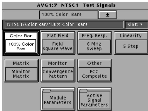
4. Each test signal icon in the Test Signals window represents one or more signals. In the following example of an NTSC test signal window, the Color Bar test signal icon is selected, and the 100% Color Bars signal is being generated.
