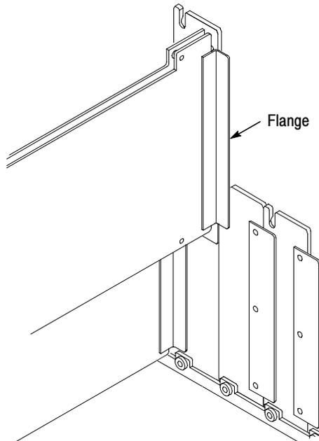
**Figure 2- 4: Module flange**
