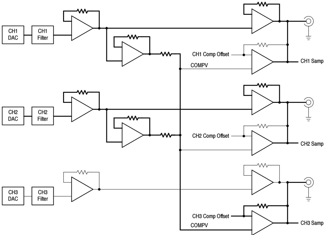
**Figure 3-3: Hardware modulated signal mode (YC composite)**
