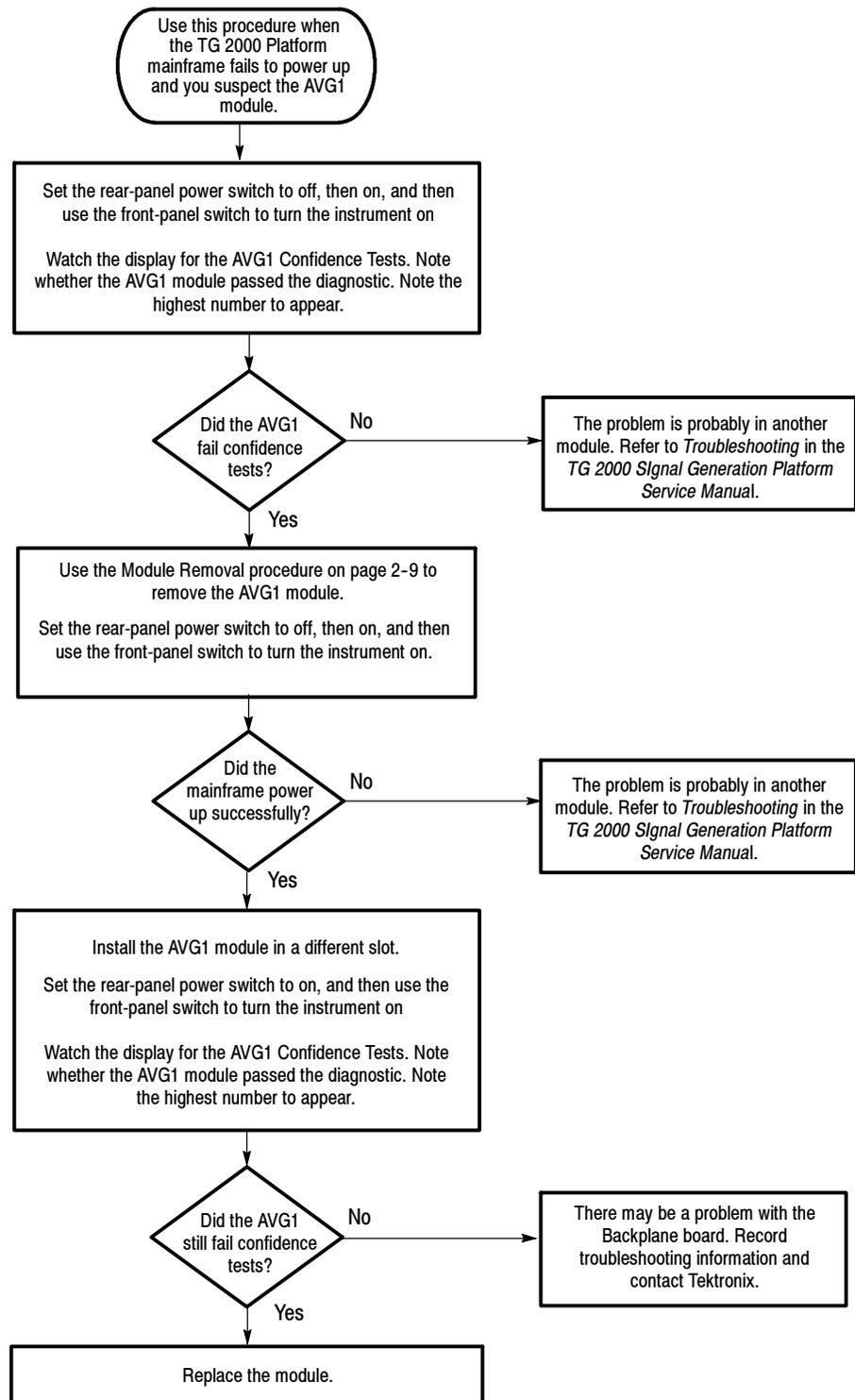
Figure 6-7: Flowchart for failure to power up
