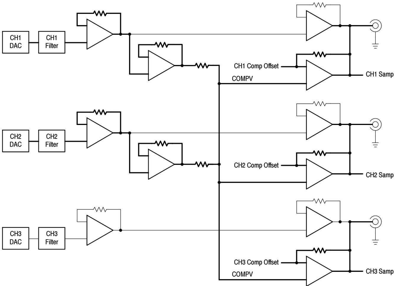
Figure 3-2: Hardware modulated signal mode (three channel composite)
