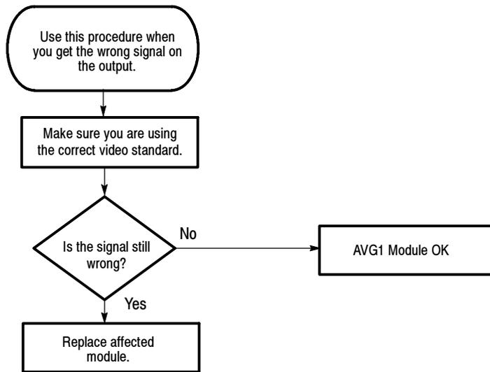
Figure 6-10: Flowchart for wrong signal on output
