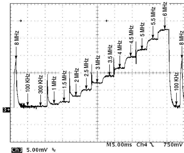
Figure 5-3: Poorly adjusted frequency response
