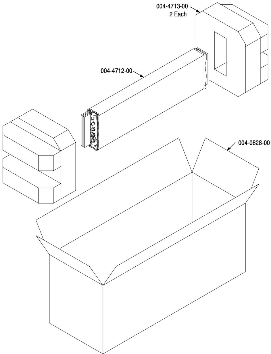
**Figure 6-2: Placing the module in the shipping carton**
