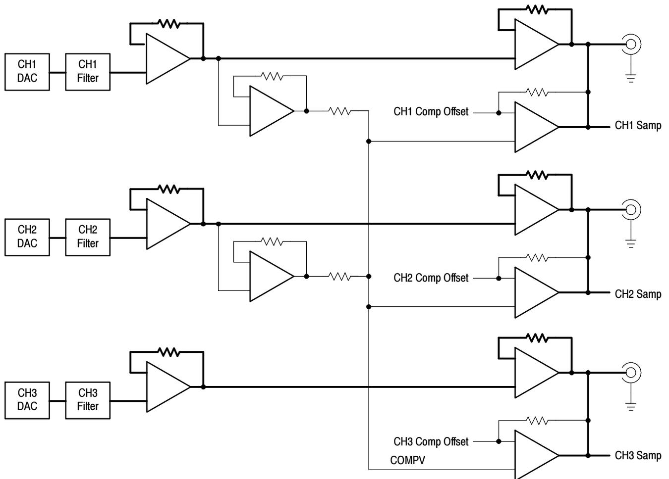
**Figure 3-4: Component and software modulated signal mode**
