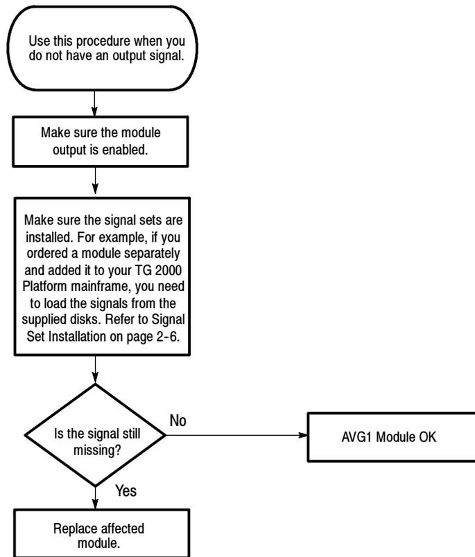
**Figure 6- 11: Flowchart for missing output signal**
