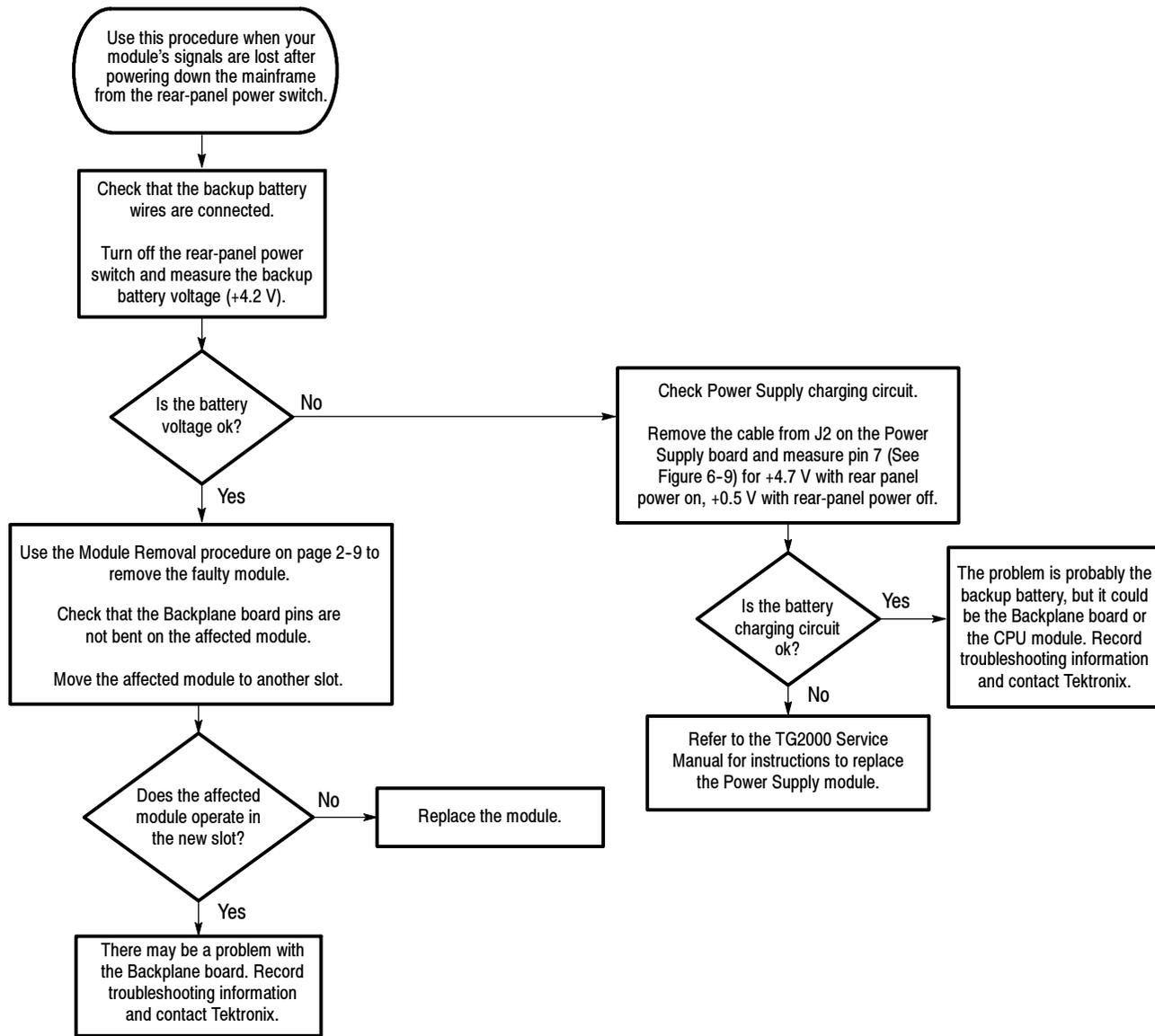
Figure 6- 8: Flowchart for signals lost after power down
