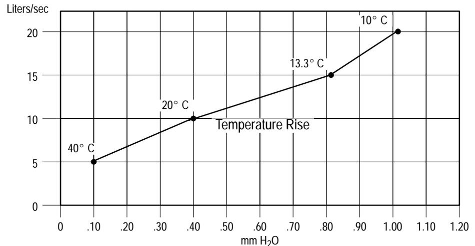
Figure 1-5: VX4351 Airflow Rate
