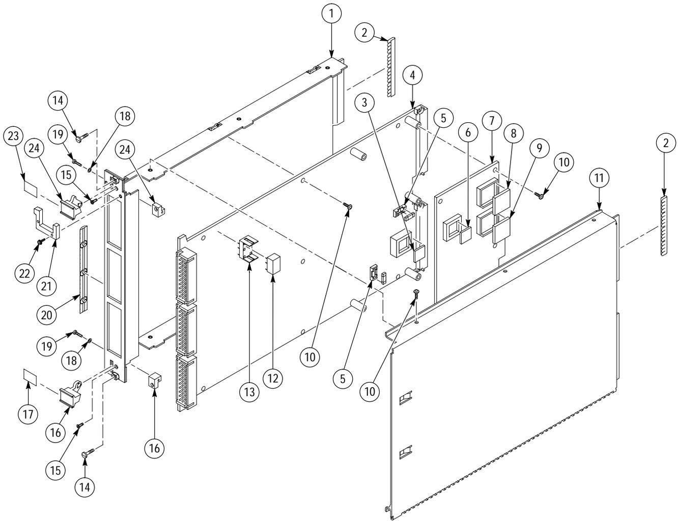
Figure F-1: VX4351 Replaceable Parts
