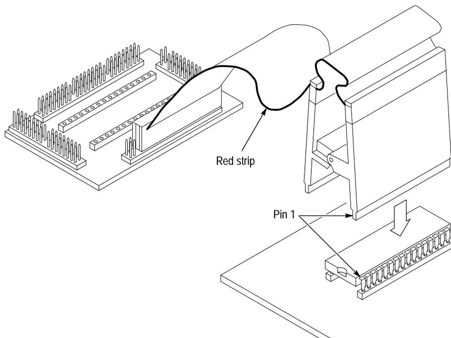
Figure 1–4: Connecting to the SUT using a DIP converter clip
