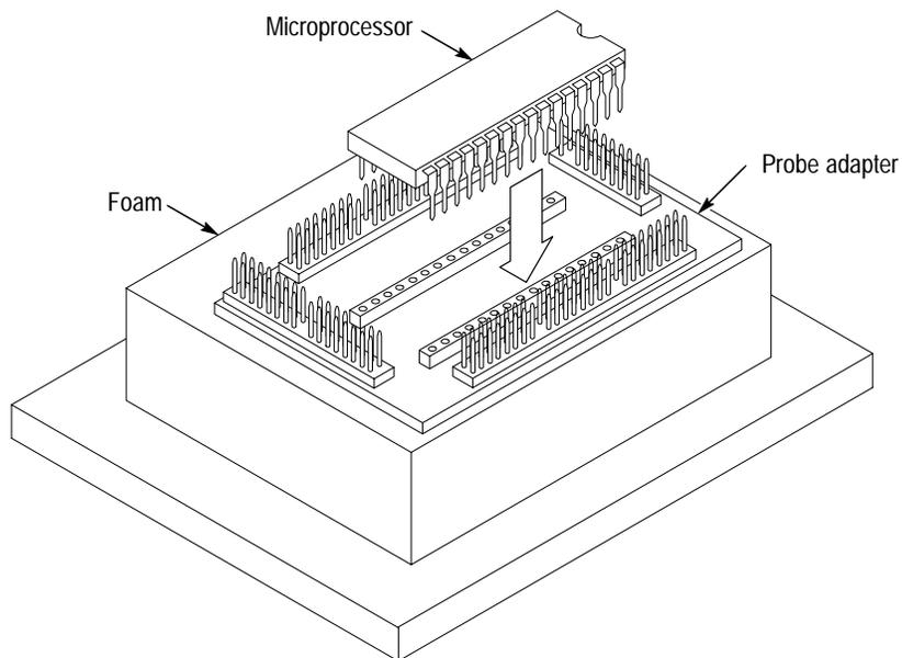
**Figure 1-1: Placing a microprocessor into a DIP probe adapter**
