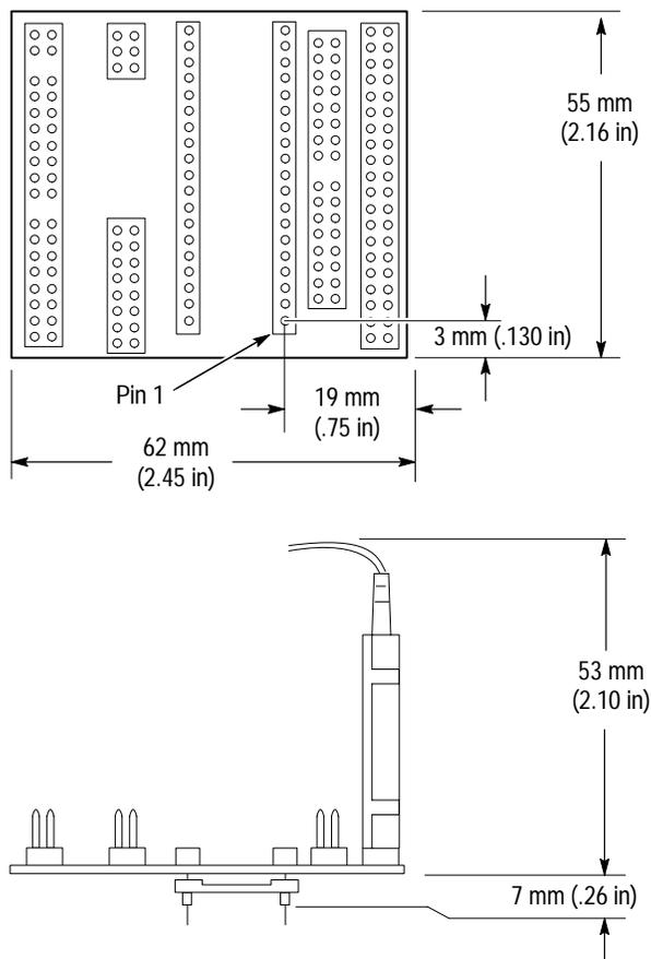
**Figure 3–1: Dimensions of the probe adapter**
