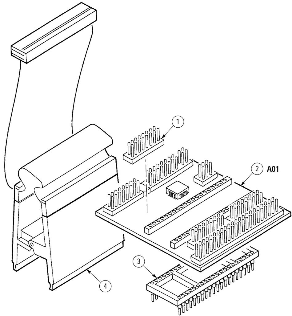
Figure 1: 8086/8088 probe adapter exploded view
