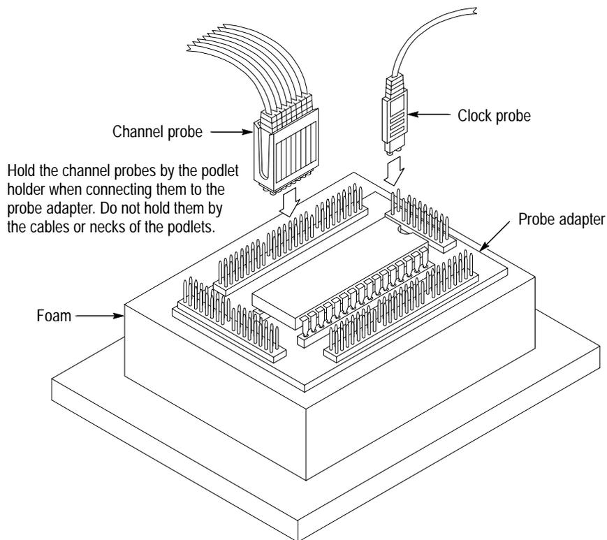
**Figure 1–2: Connecting probes to a DIP probe adapter**
