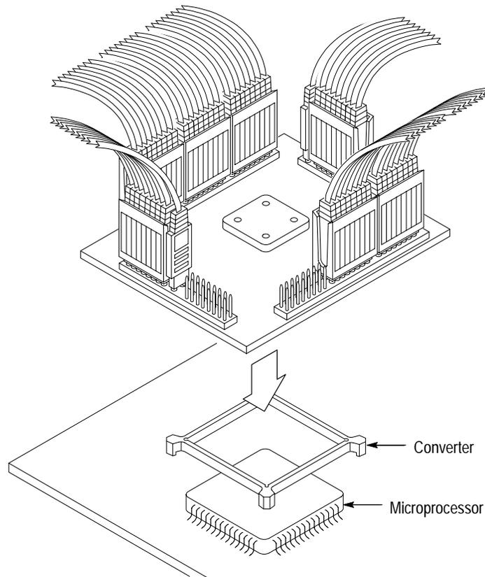
**Figure 1-10: Placing a CQFP probe adapter onto the SUT**
