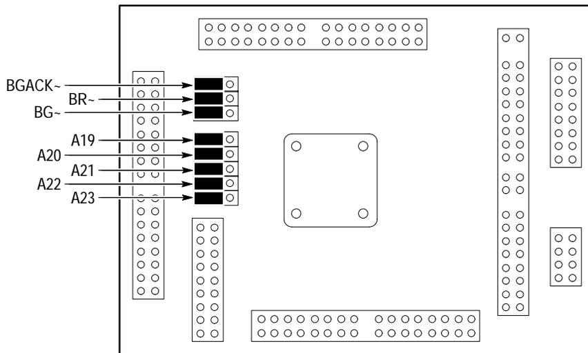
**Figure 1–1: Jumper locations on the 68331/332 QFP probe adapter**
