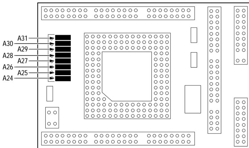
Figure 3–2: Jumper locations on the 68340 PGA probe adapter
