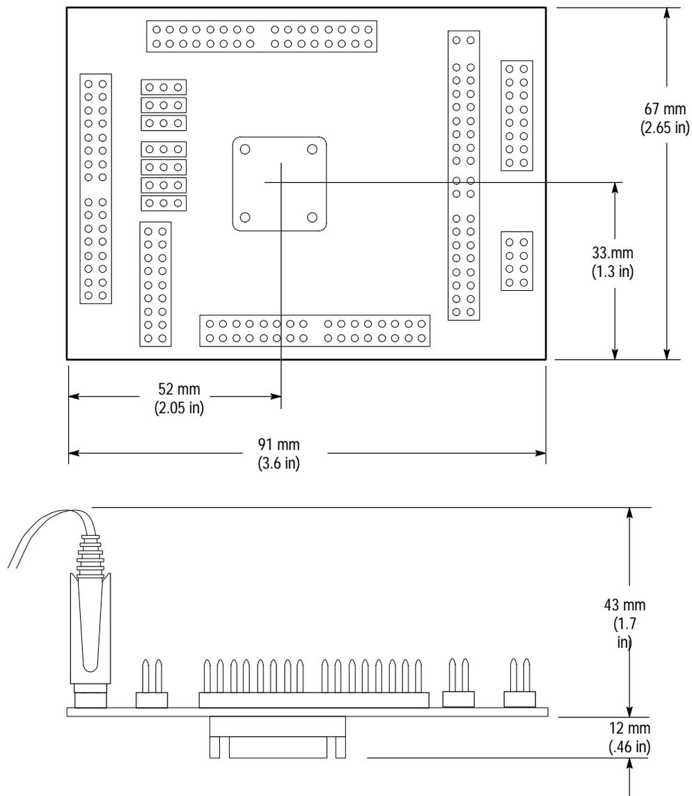
Figure 3–4: Minimum clearance of the 68331/332 QFP probe adapter
