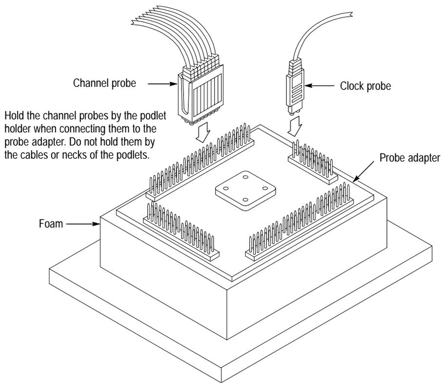
**Figure 1–7: Connecting probes to a PQFP probe adapter**
