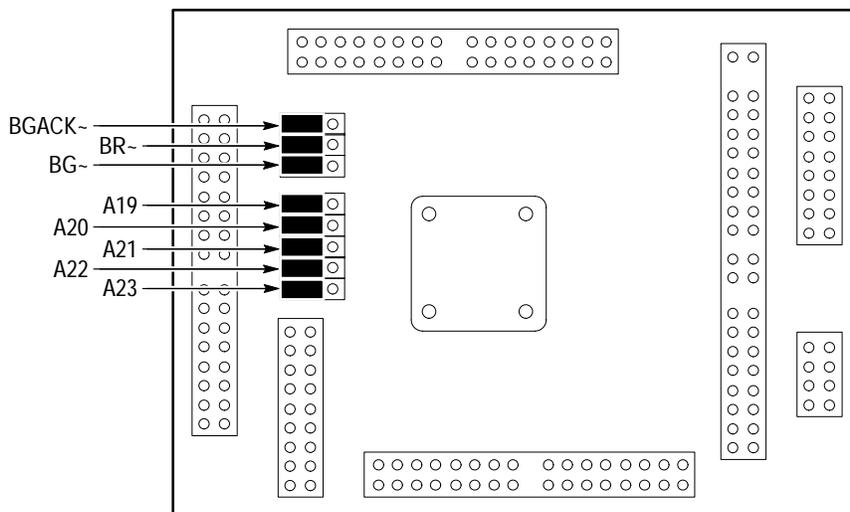
Figure 3–1: Jumper locations on the 68331/332 QFP probe adapter
