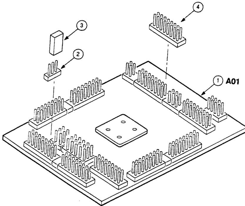
Figure 1: 68331/332 QFP probe adapter exploded view
