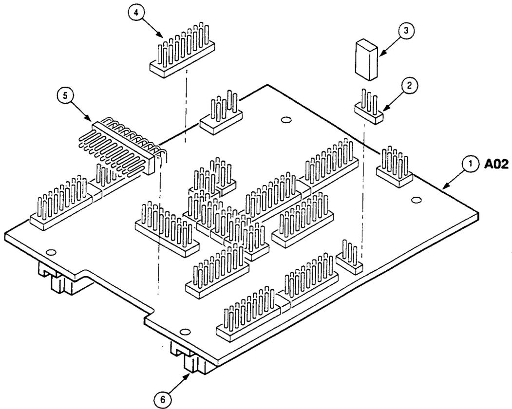
Figure 2: 68331/332 Evaluation Board probe adapter exploded view
