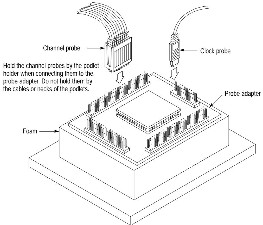
**Figure 1-5: Connecting probes to a PGA probe adapter**
