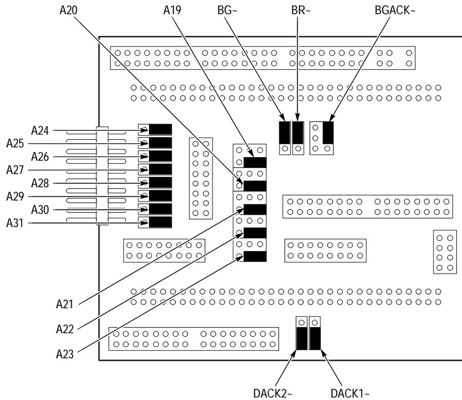
Figure 3–3: Jumper locations on the 68331/332 Evaluation Board probe adapter
