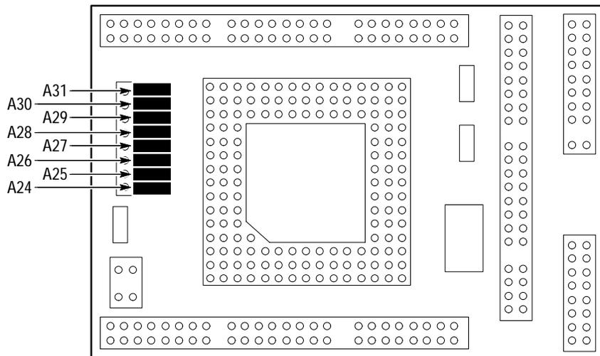
**Figure 1–2: Jumper locations on the 68340 PGA probe adapter**
