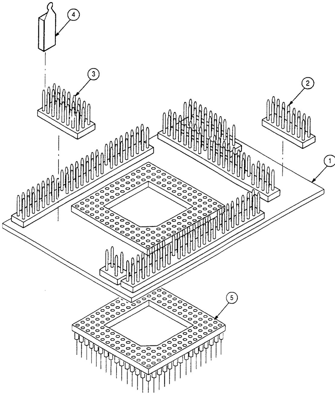
Figure 3: 68340 PGA probe adapter exploded view
