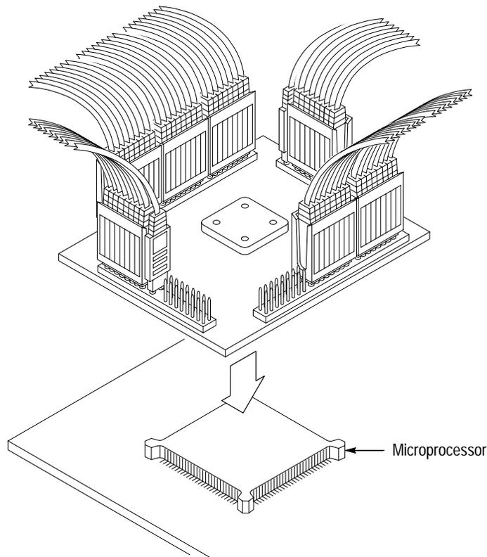
Figure 1-8: Placing a PQFP probe adapter onto the SUT
