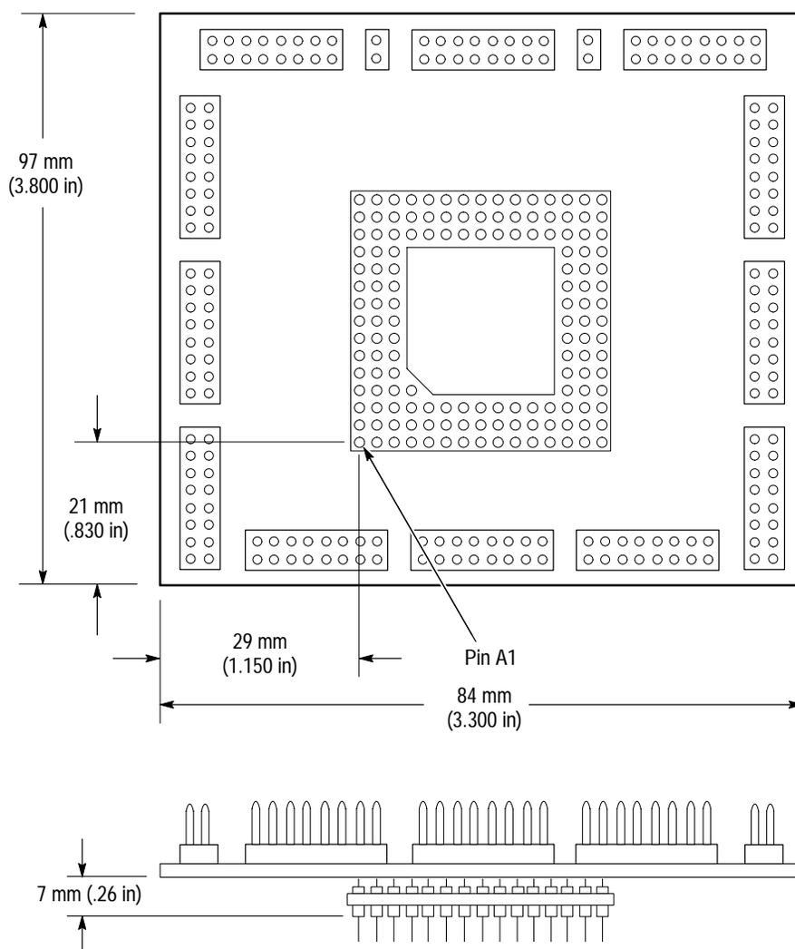
**Figure 3–1: Dimensions of the probe adapter**
