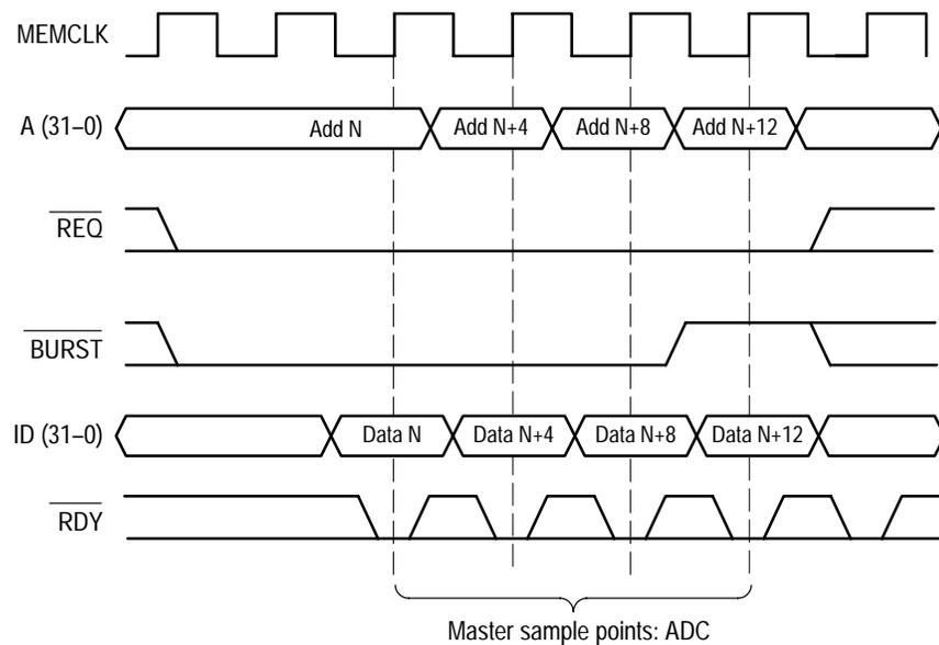
Figure 3–3: 29030/35/40 bus timing: Burst Access
