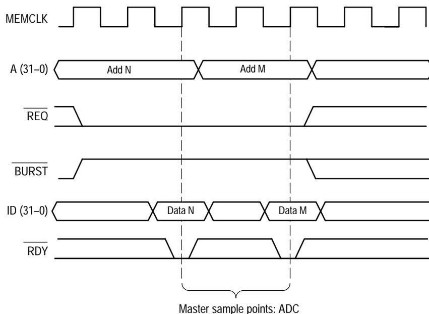
Figure 3–2: 29030/35/40 bus timing: Simple Access
