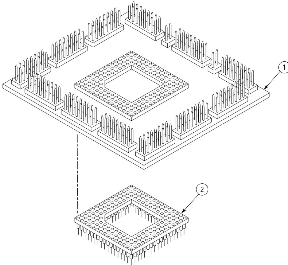
**Figure 1: 29030/35/40 probe adapter exploded view**
