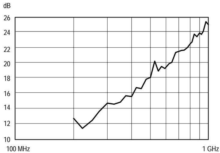
Figure 3–2: Sample plot of log periodic antenna factors
