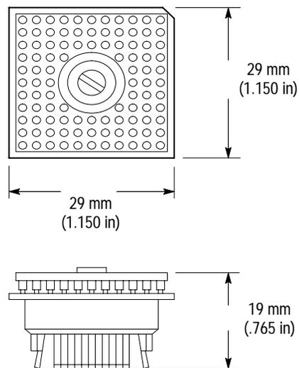
Figure 3-2: Dimensions of the test clip
