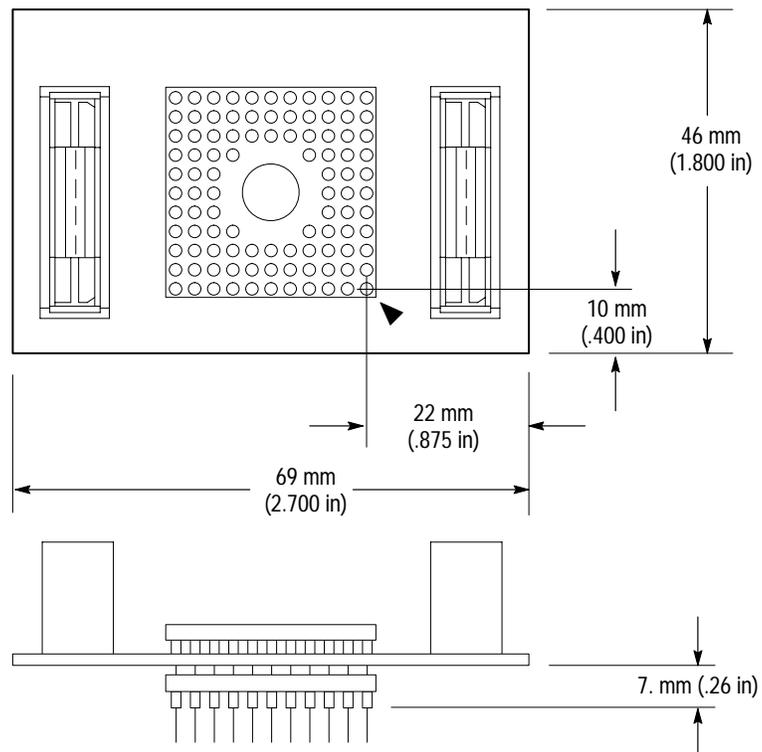
Figure 3-1: Dimensions of the probe adapter
