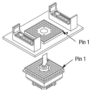
**Figure 1–1: Connecting the test clip to the probe adapter**
