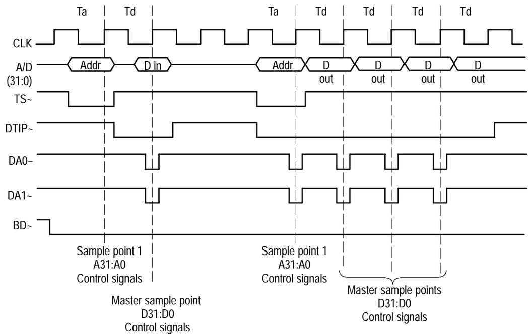
Figure 2-1: MCF5202/03 bus timing
