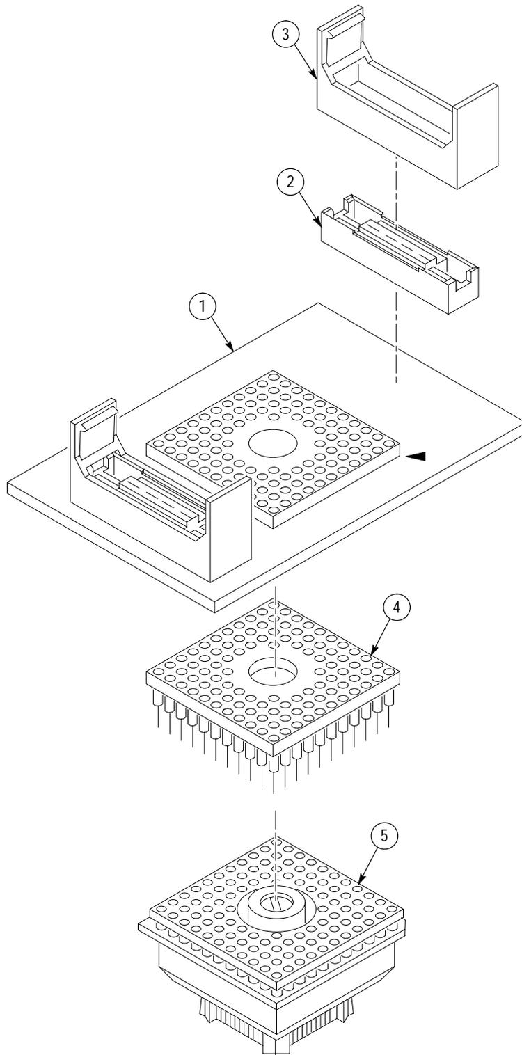
Figure 1: MCF5202/03 probe adapter exploded view
