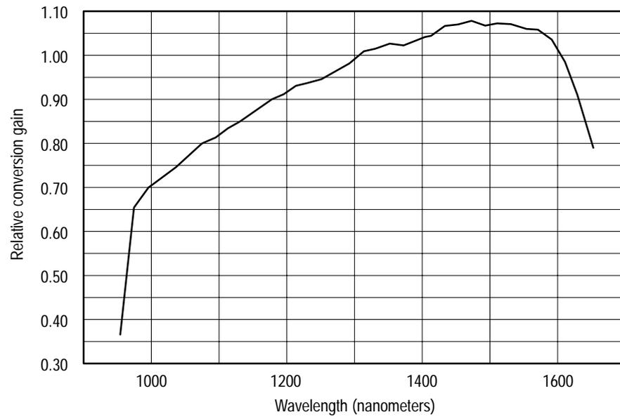
**Figure 5: SD-44 relative responsivity (normalized to 1310 nm)**
