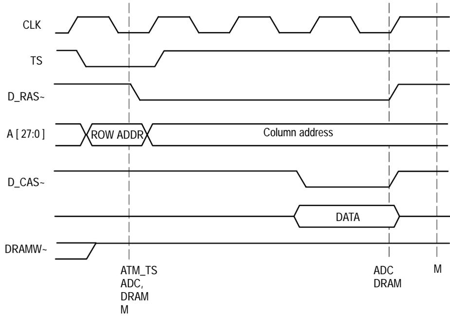
**Figure 2-2:** Byte Read transfer in normal mode with 8-bit NON EDO Dram
