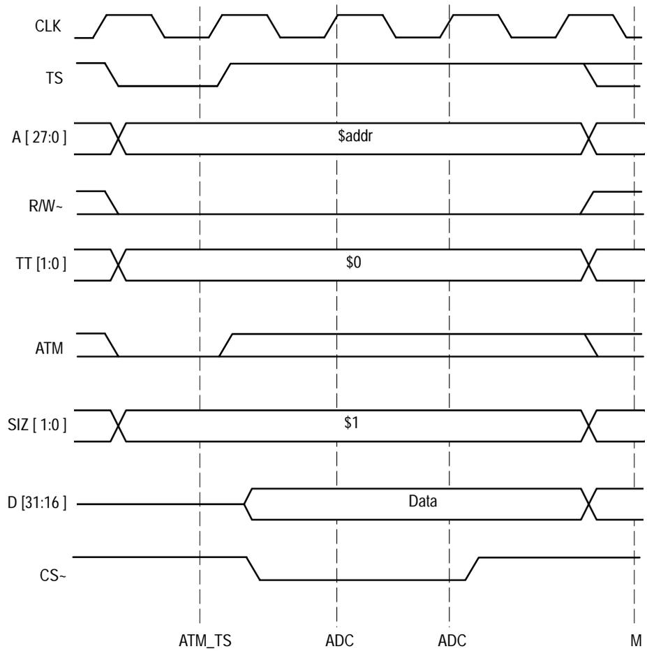
**Figure 2-1:** Byte Write Transfer from an 8-bit port.
