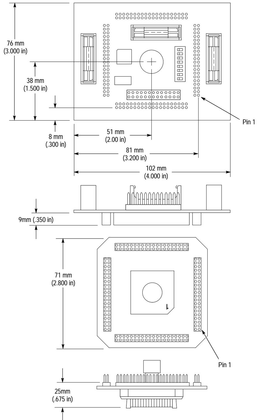
Figure 3-1: Dimensions of the probe adapter
