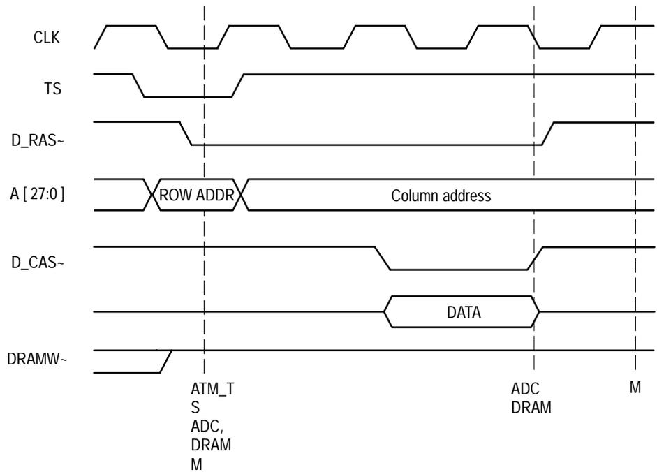
**Figure 2-3:** Byte Read transfer in normal mode with 8-bit EDO Dram
