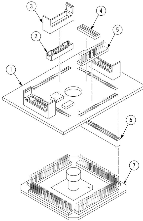
Figure 6-1: MCF5206 probe adapter exploded view
