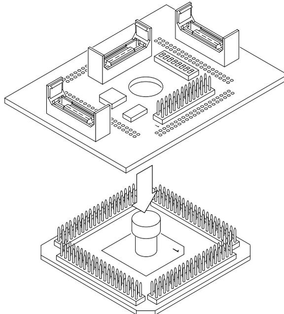
Figure 1-1: Connecting the test clip to the probe adapter
