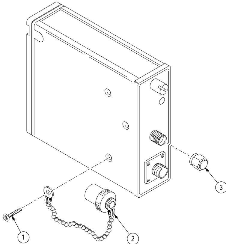
Figure 8: SD-43 replaceable parts
