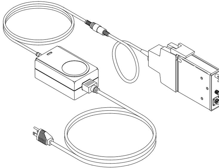
**Figure 5: Installation with optional power supply kit**
