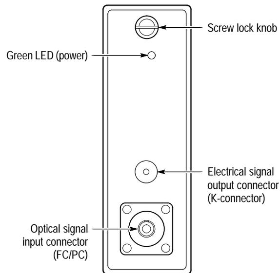
**Figure 1: SD-43 front panel**
