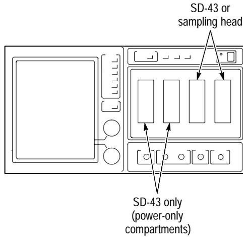
**Figure 4: Front panel compartments in a CSA 803 Communications Signal Analyzer**
